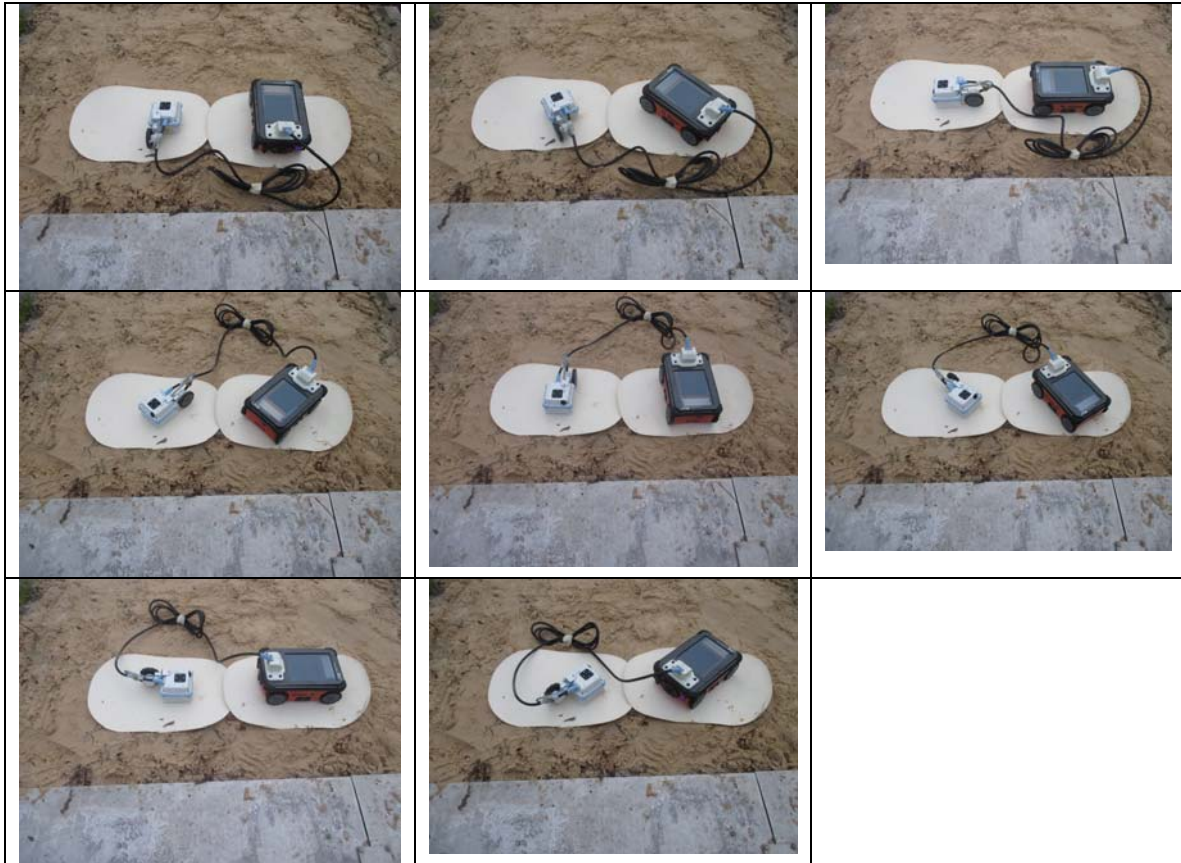
EUT Positions with 45 Degree Interval
