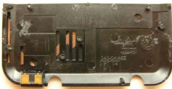
Fig 10 –Antenna module/cover: rear view (Integral 850/900/1800/1900 antennas)
