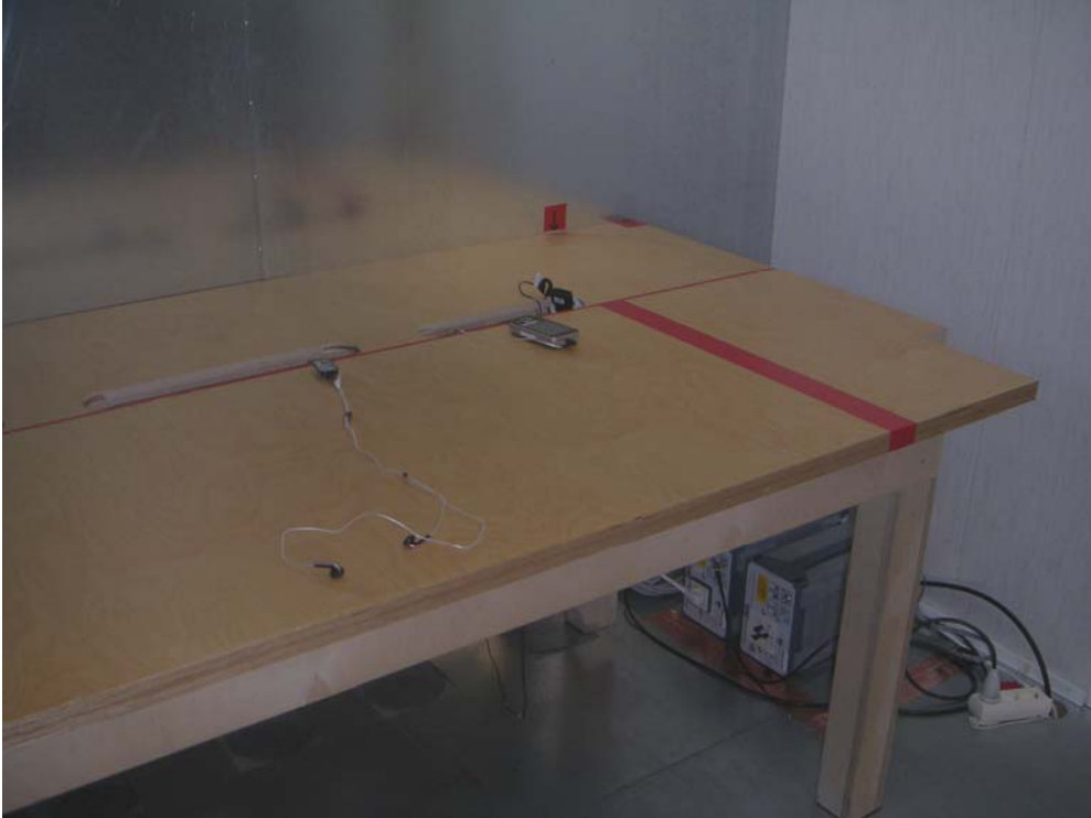
Picture 3 AC powerline conducted emission measurement
