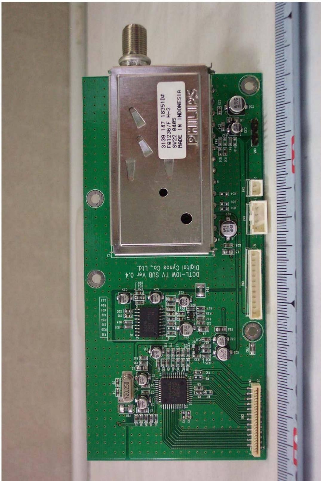
● Rear View of TV Tuner Sub Board
