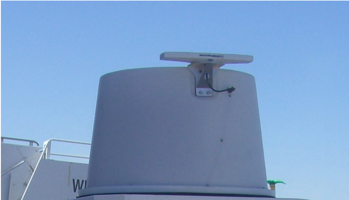
Radar covered by protective Radome
