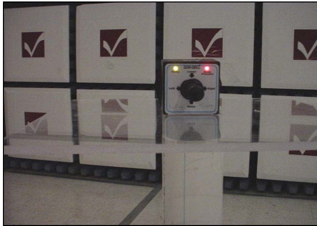
View of the EUT in Vertical Orientation This orientation had the highest measured emissions.
