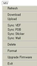
10) **Upgrade Firmware**: Download the new firmware software from the PC. Old firmware will be stored in the folder where ‘MagicTools’ installed. Performing this function erases all contents in flash memory, so read all precautions described in “Format”. Only use this function to download official upgrade firmware from MagicEyes.
