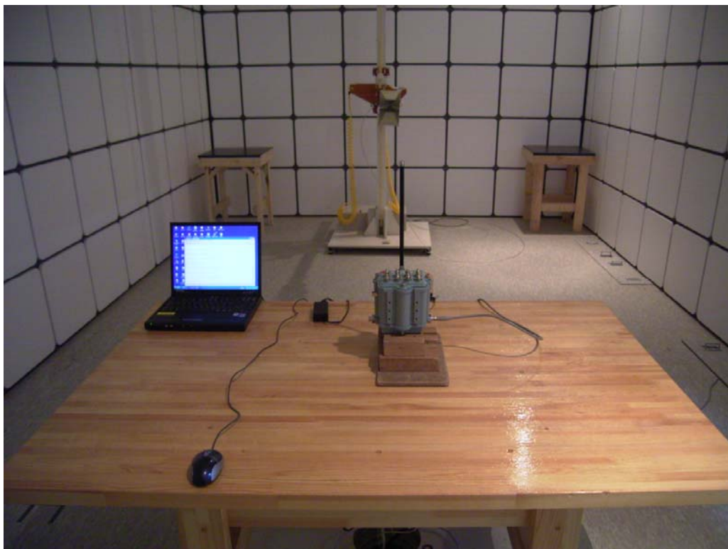
Radiated Emissions(1000MHz~18000MHz)- Front View
