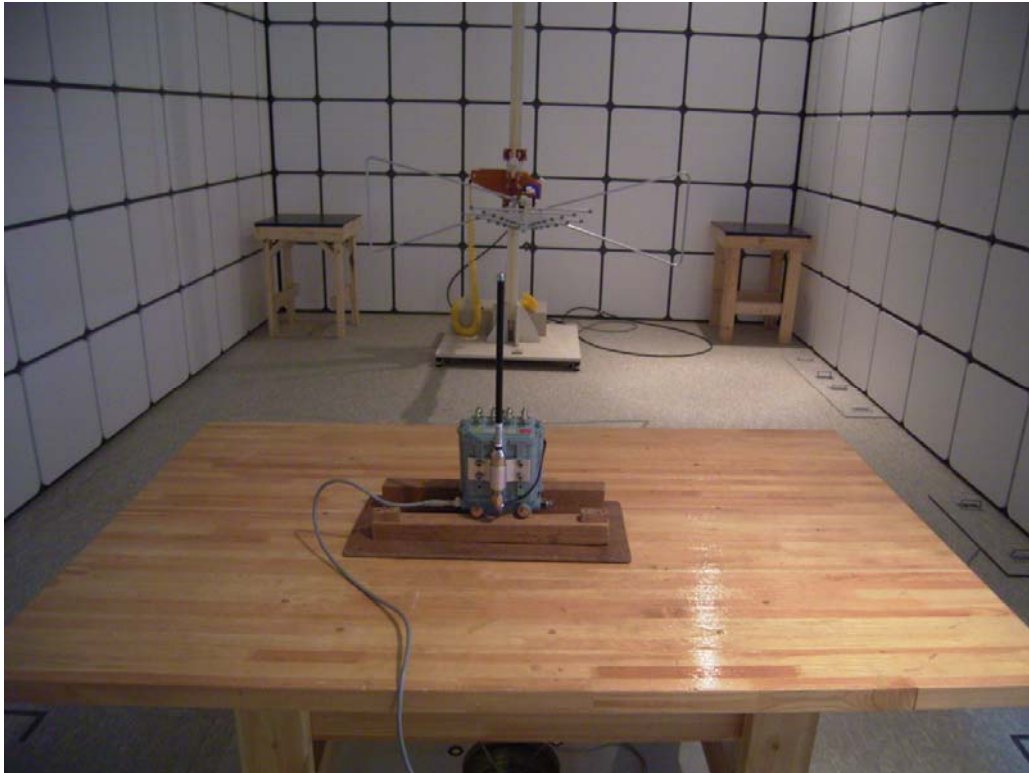
Radiated Emissions(30MHz~1000MHz)- Front View
