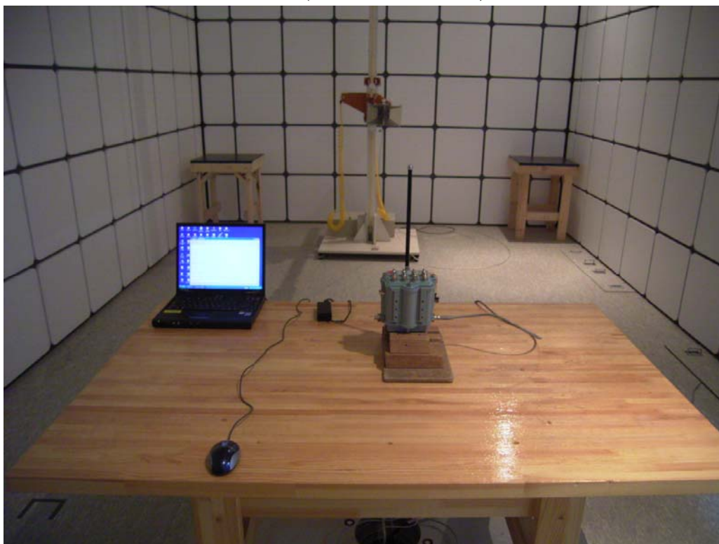
Radiated Emissions(1000MHz~18000MHz)- Rear View
