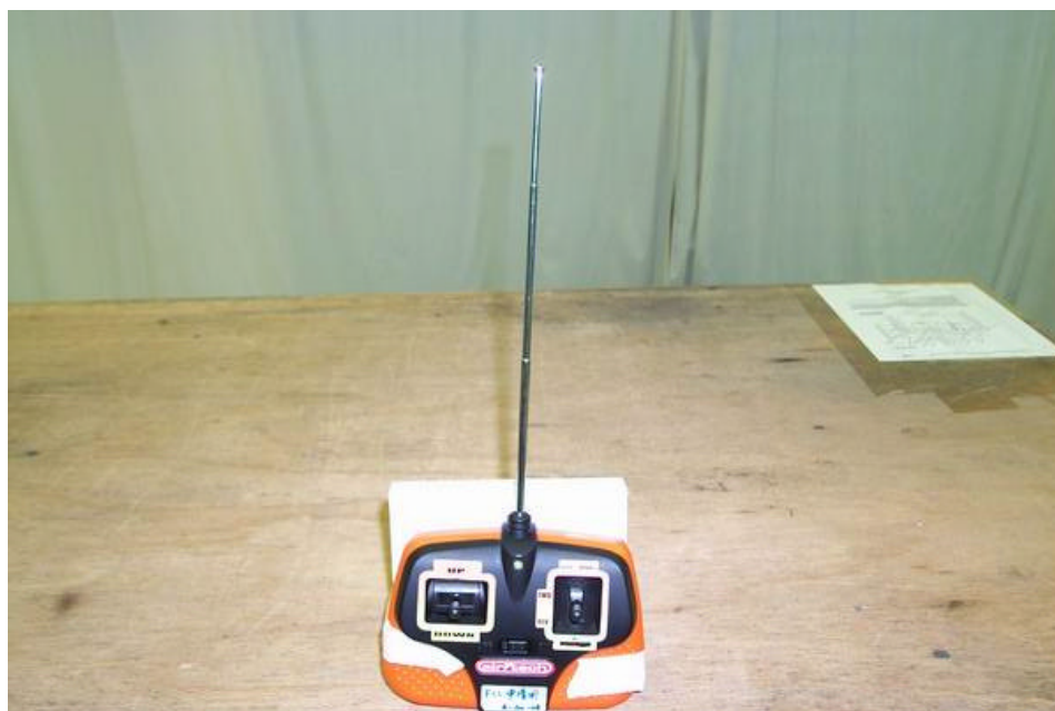
Figure 3.1 Radiated Test Setup, position 1-X
