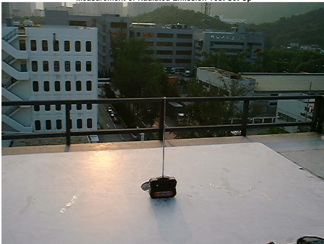
Measurement of Radiated Emission Test Set Up
