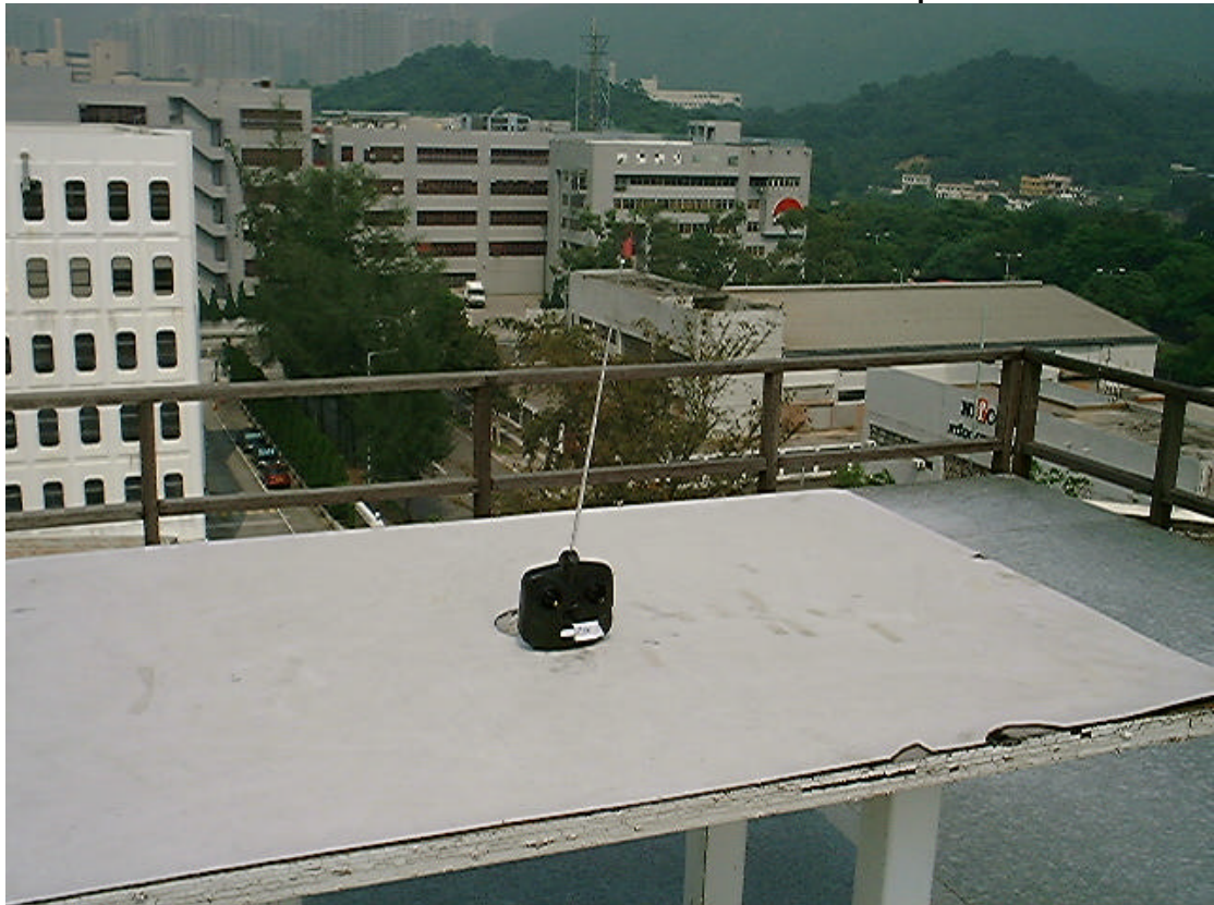
Measurement of Radiated Emission Test Set Up
