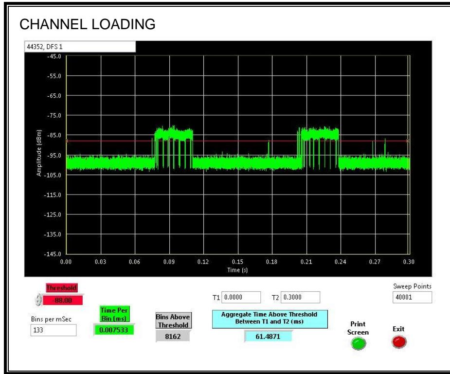
The level of traffic loading on the channel by the EUT is 20.495%
