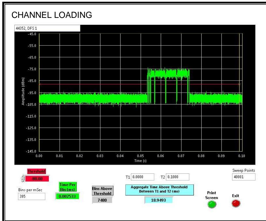
The level of traffic loading on the channel by the EUT is 18.9493%
