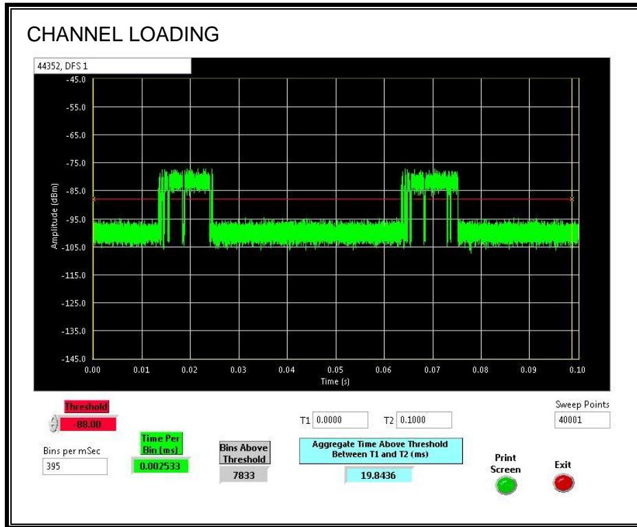
The level of traffic loading on the channel by the EUT is 19.8436%
