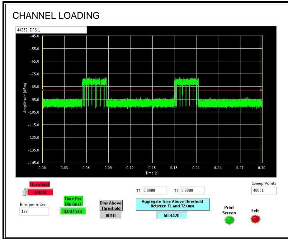
The level of traffic loading on the channel by the EUT is 20.114%
