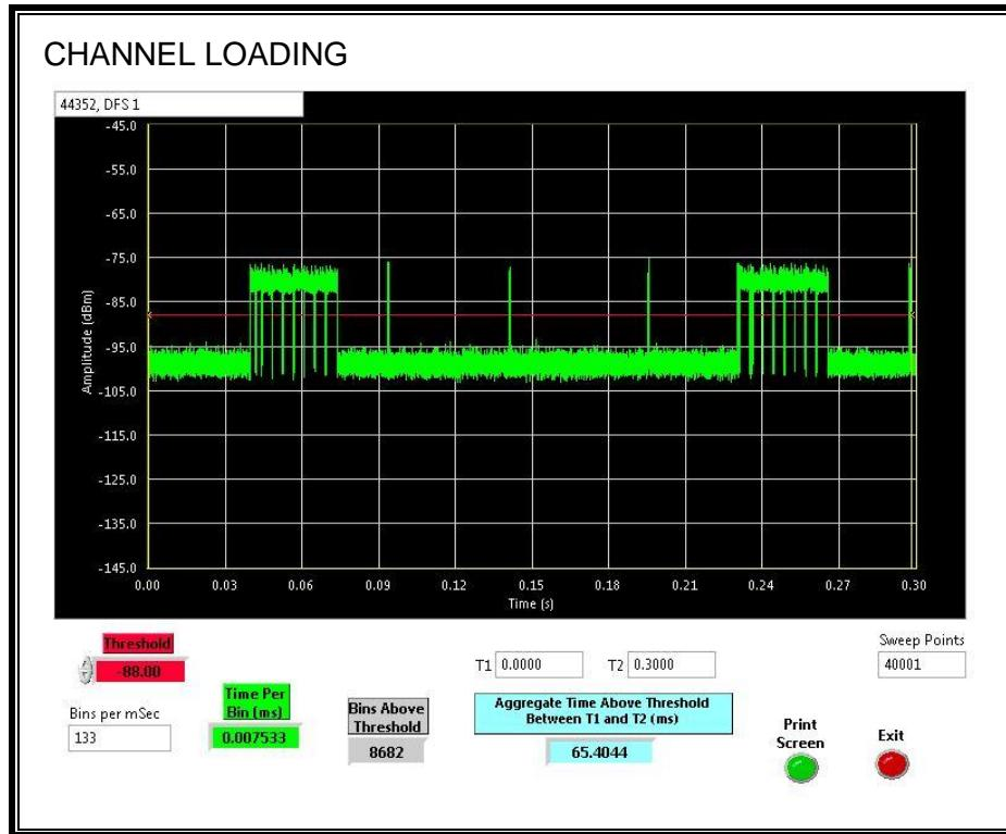
The level of traffic loading on the channel by the EUT is 21.8%
