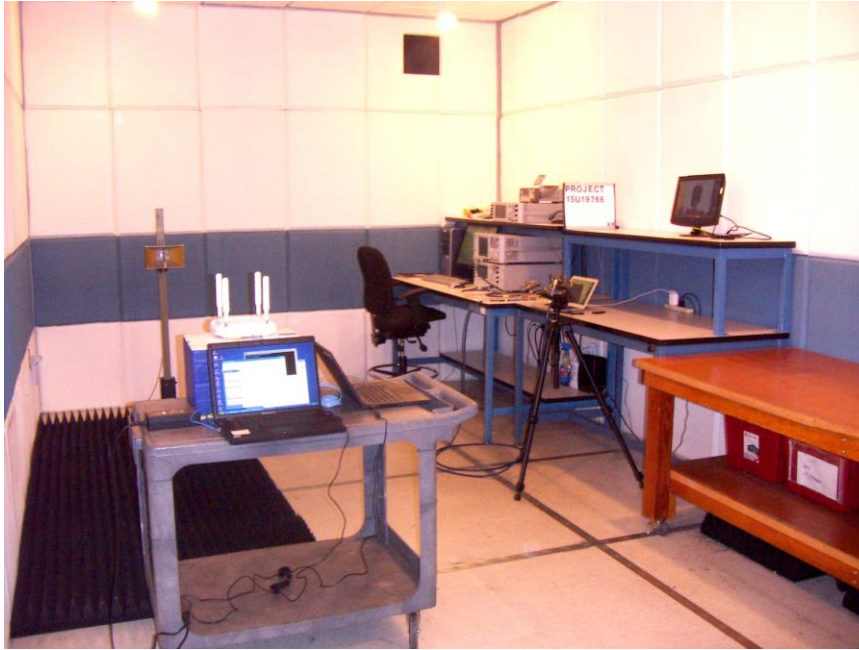
DFS FRONT PHOTO (CLIENT-TO-CLIENT COMMUNICATIONS MODE SETUP)
