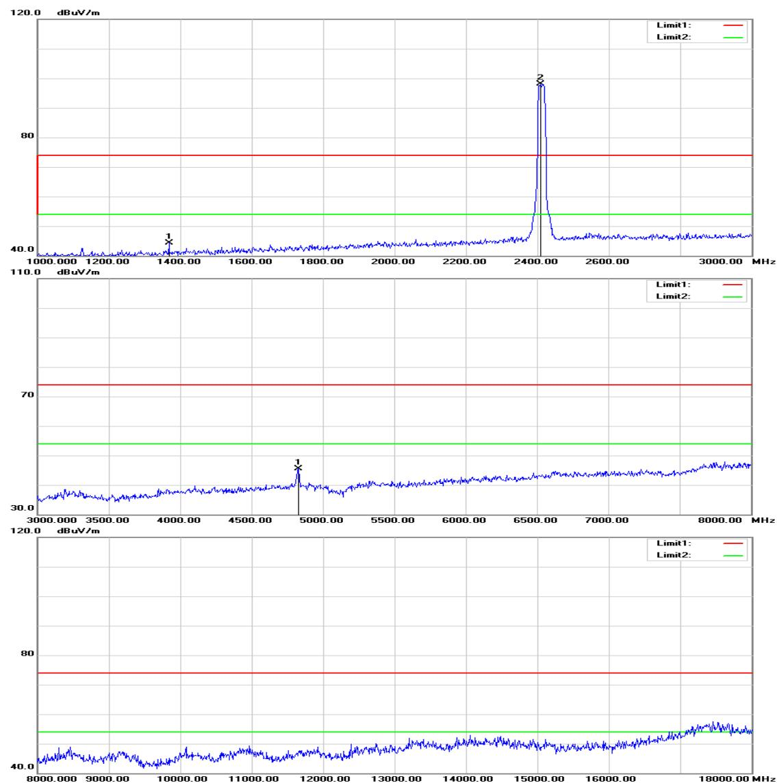
**Operation Mode:** TX / IEEE 802.11g / CH Low**Test Date:** August 19, 2015**Temperature:** 27°C**Tested by:** Owen Wu**Humidity:** 53% RH**Polarity:** Ver. / Hor.
