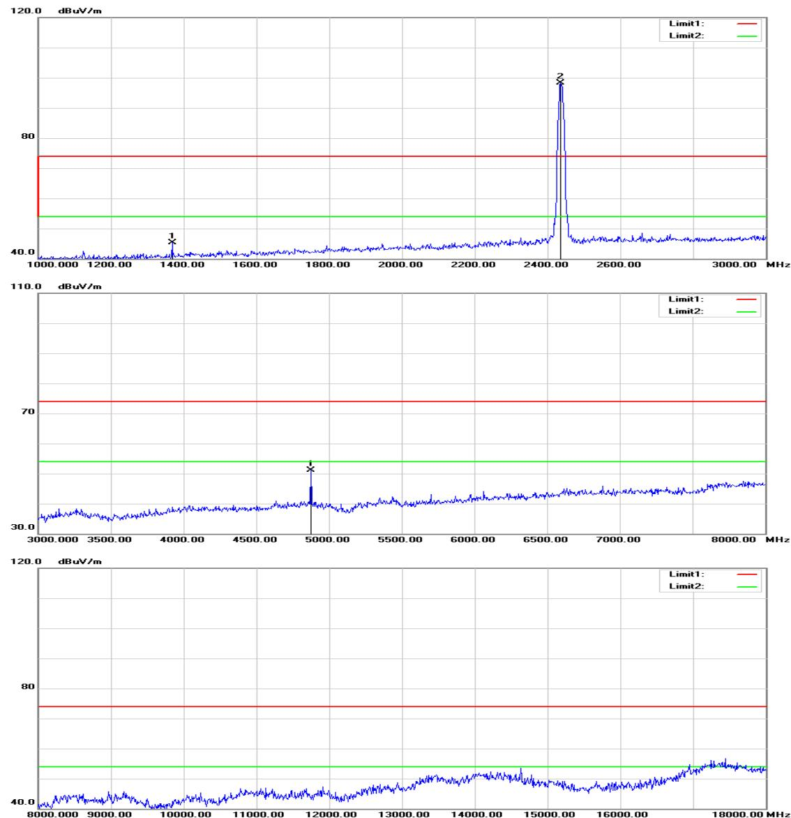
**Operation Mode:** TX / IEEE 802.11b / CH Mid**Test Date:** August 19, 2015**Temperature:** 27°C**Tested by:** Owen Wu**Humidity:** 53% RH**Polarity:** Ver. / Hor.
