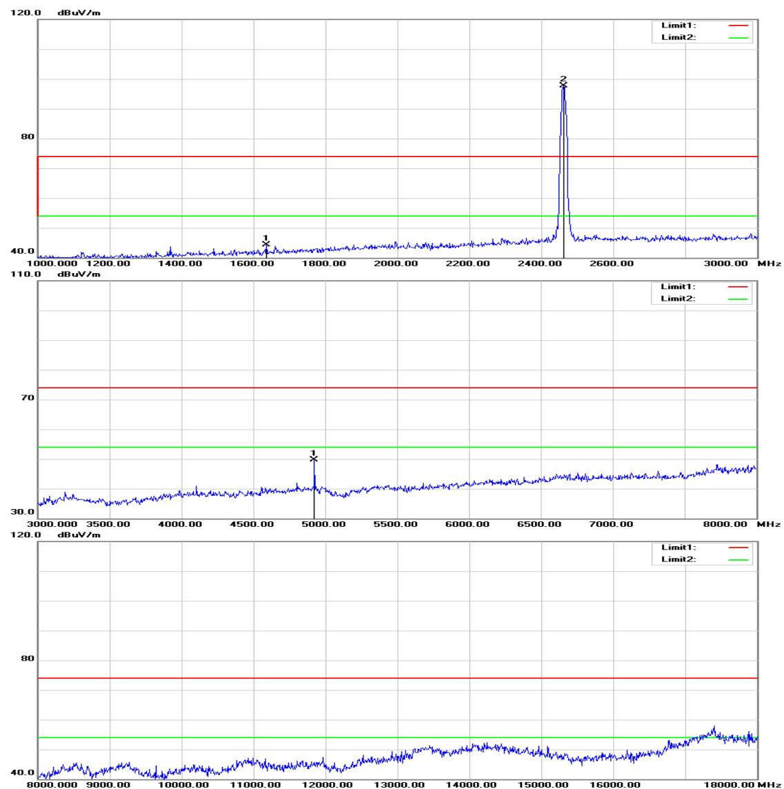
**Operation Mode:** TX / IEEE 802.11b / CH High**Test Date:** August 19, 2015**Temperature:** 27°C**Tested by:** Owen Wu**Humidity:** 53% RH**Polarity:** Ver. / Hor.
