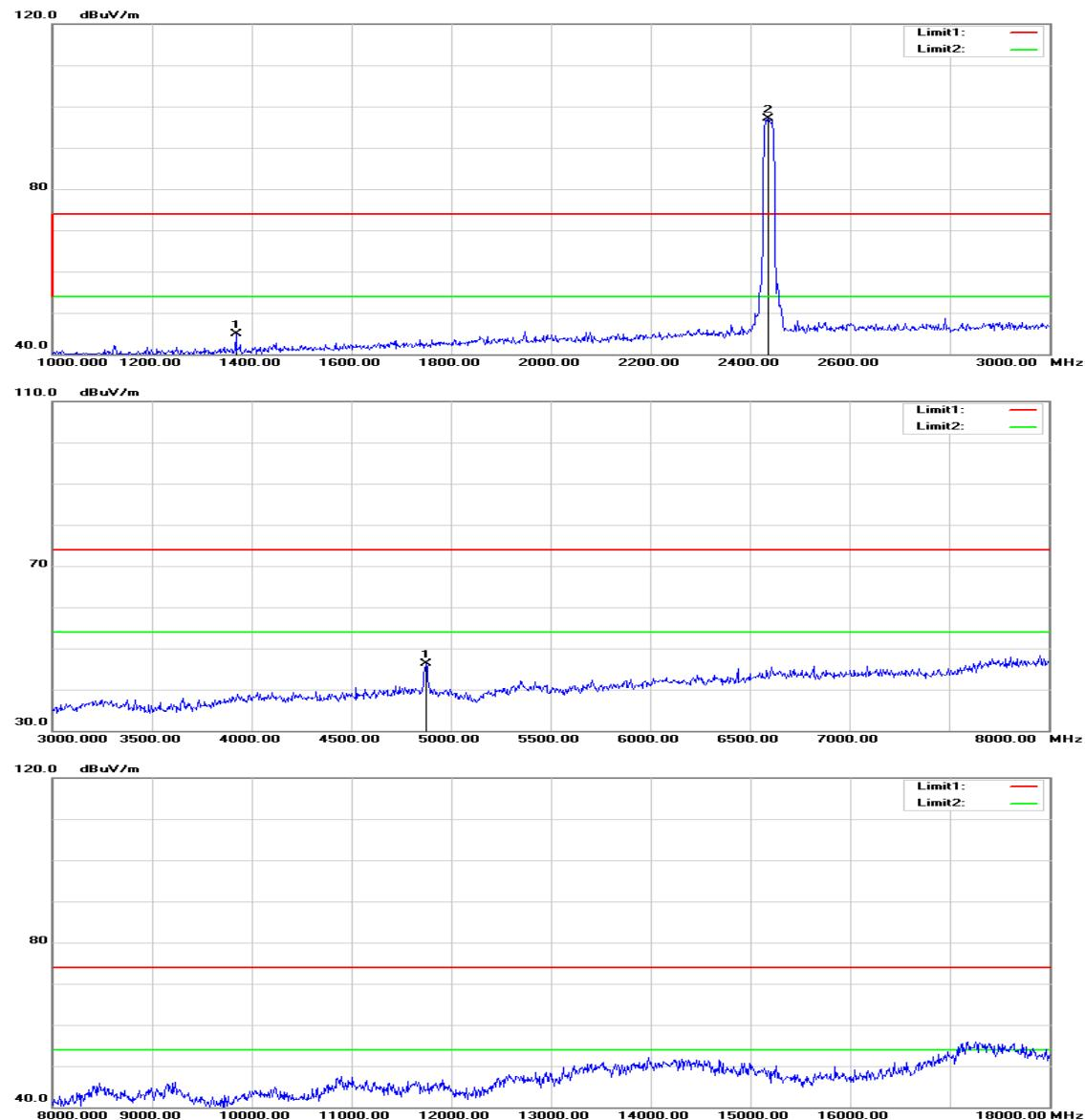
**Operation Mode:** TX / IEEE 802.11g / CH Mid**Test Date:** August 19, 2015**Temperature:** 27°C**Tested by:** Owen Wu**Humidity:** 53% RH**Polarity:** Ver. / Hor.
