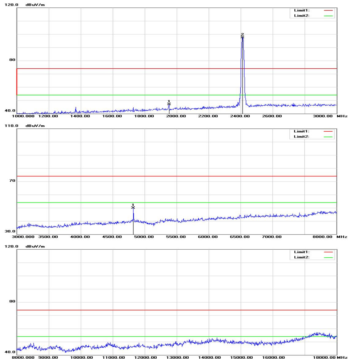
**Above 1 GHz****Operation Mode:** TX / IEEE 802.11b / CH Low**Test Date:** August 19, 2015**Temperature:** 27°C**Tested by:** Owen Wu**Humidity:** 53% RH**Polarity:** Ver. / Hor.
