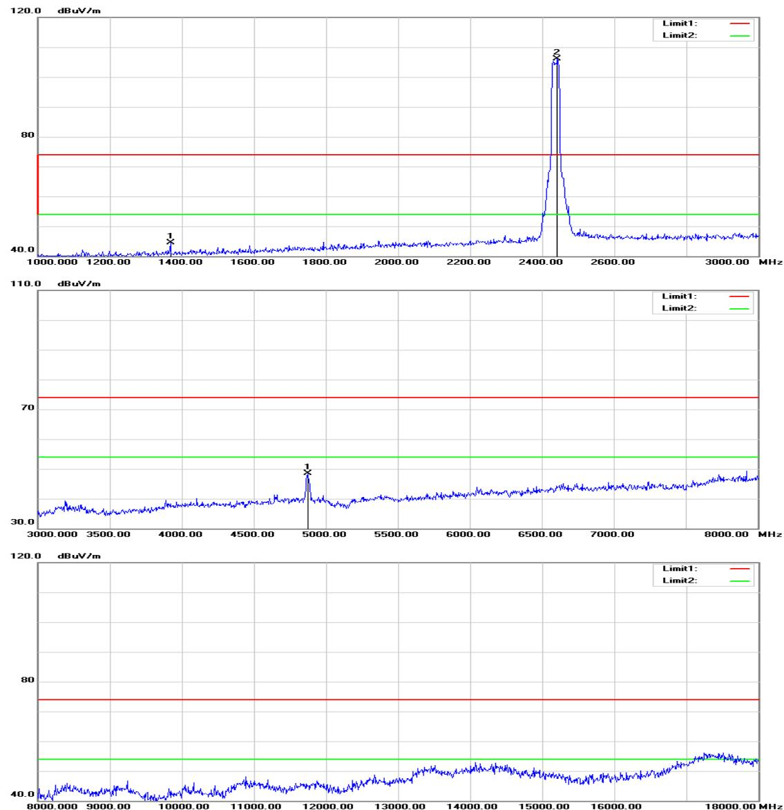
**Operation Mode:** TX / IEEE 802.11n HT 20 MHz mode / CH Mid **Test Date:** August 19, 2015**Temperature:** 27°C**Tested by:** Owen Wu**Humidity:** 53% RH**Polarity:** Ver. / Hor.
