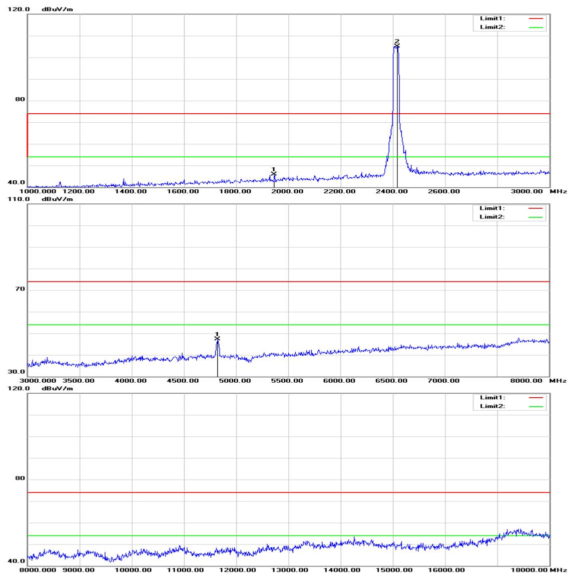
**Operation Mode:** TX / IEEE 802.11n HT 20 MHz mode / CH Low **Test Date:** August 19, 2015
