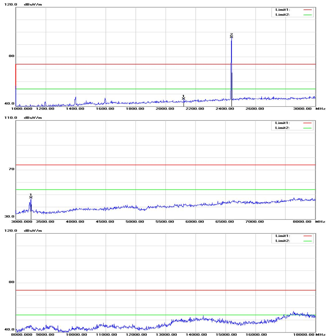
**Operation Mode:** GFSK / TX / CH Mid    **Test Date:** August 19, 2015
