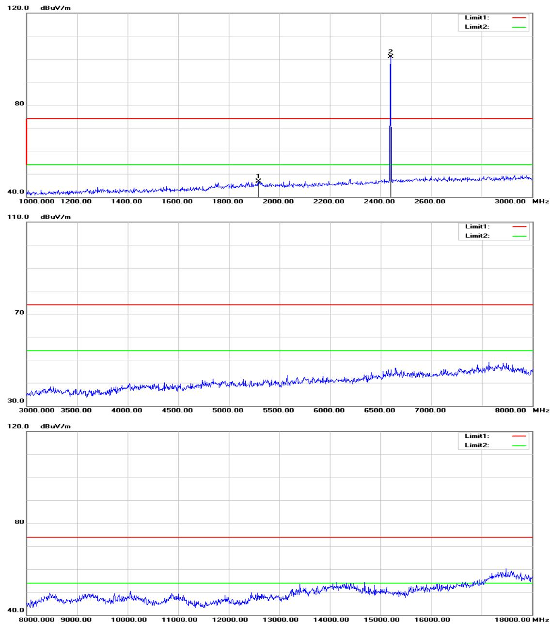
**Operation Mode:** GFSK / TX / CH Mid    **Test Date:** August 1, 2015
