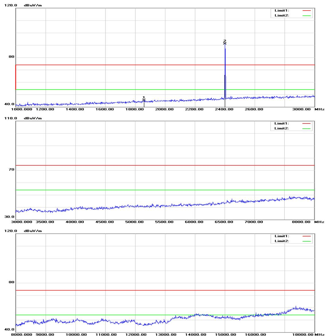
**Above 1 GHz****Operation Mode:** TX / GFSK / DH5 / CH Low**Test Date:** July 29, 2015**Temperature:** 27°C**Tested by:** Owen Wu**Humidity:** 53 % RH**Polarity:** Ver. / Hor.
