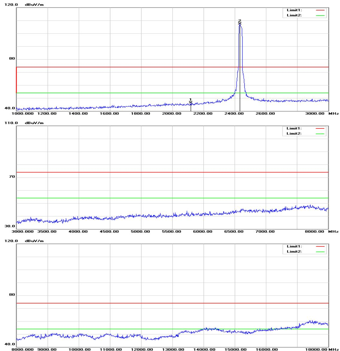
**Operation Mode:** TX / IEEE 802.11n HT 20 MHz mode / CH Mid **Test Date:** July 29, 2015
