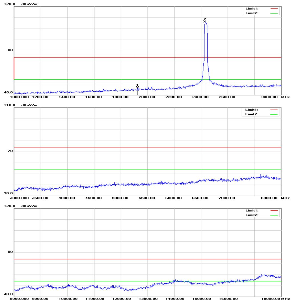
**Operation Mode:** TX / IEEE 802.11g / CH Mid**Test Date:** July 29, 2015**Temperature:** 27°C**Tested by:** Owen Wu**Humidity:** 53% RH**Polarity:** Ver. / Hor.
