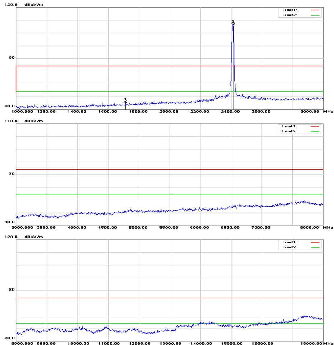
**Above 1 GHz****Operation Mode:** TX / IEEE 802.11b / CH Low**Test Date:** July 29, 2015**Temperature:** 27°C**Tested by:** Owen Wu**Humidity:** 53% RH**Polarity:** Ver. / Hor.
