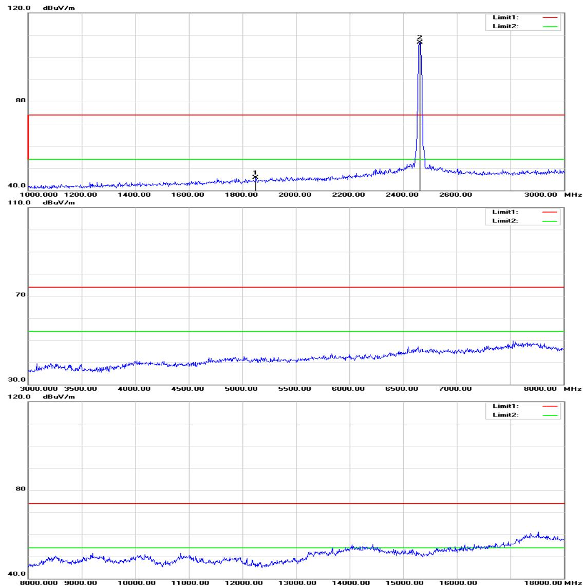
**Operation Mode:** TX / IEEE 802.11b / CH High**Test Date:** July 29, 2015**Temperature:** 27°C**Tested by:** Owen Wu**Humidity:** 53% RH**Polarity:** Ver. / Hor.
