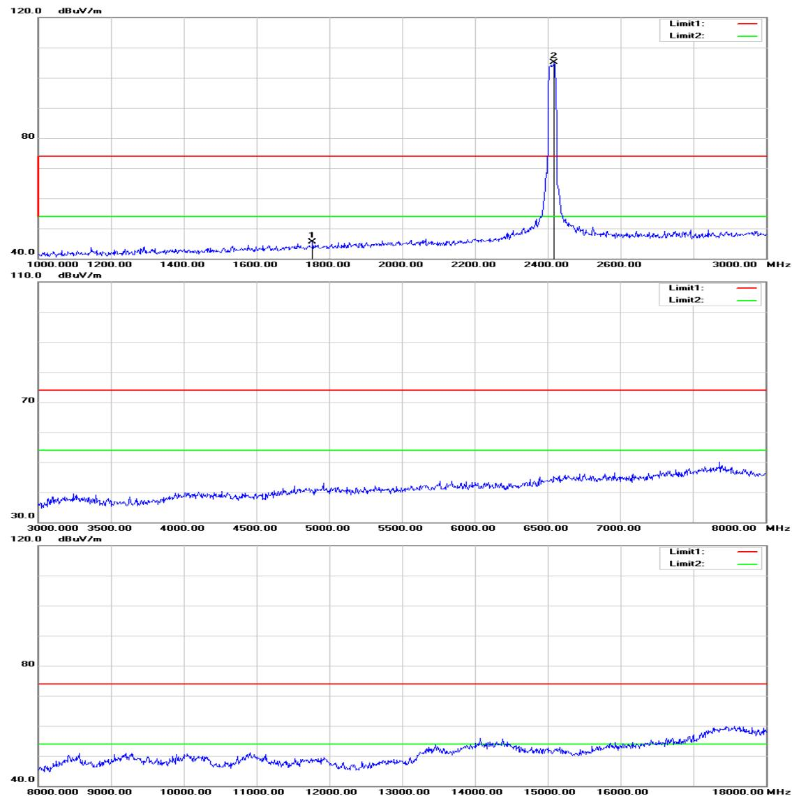
**Operation Mode:** TX / IEEE 802.11g / CH Low**Test Date:** July 29, 2015**Temperature:** 27°C**Tested by:** Owen Wu**Humidity:** 53% RH**Polarity:** Ver. / Hor.
