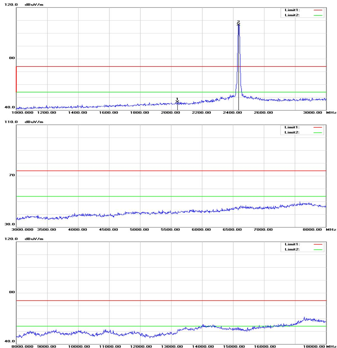
**Operation Mode:** TX / IEEE 802.11b / CH Mid**Test Date:** July 29, 2015**Temperature:** 27°C**Tested by:** Owen Wu**Humidity:** 53% RH**Polarity:** Ver. / Hor.
