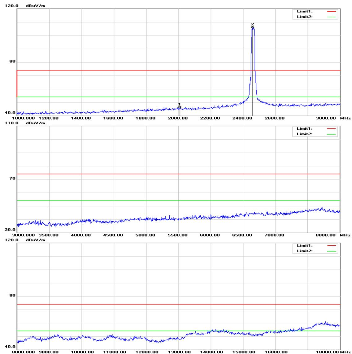
**Operation Mode:** TX / IEEE 802.11g / CH High**Test Date:** July 29, 2015**Temperature:** 27°C**Tested by:** Owen Wu**Humidity:** 53% RH**Polarity:** Ver. / Hor.
