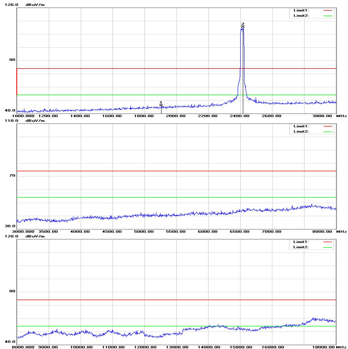
**Operation Mode:** TX / IEEE 802.11n HT 20 MHz mode / CH Low **Test Date:** July 29, 2015
