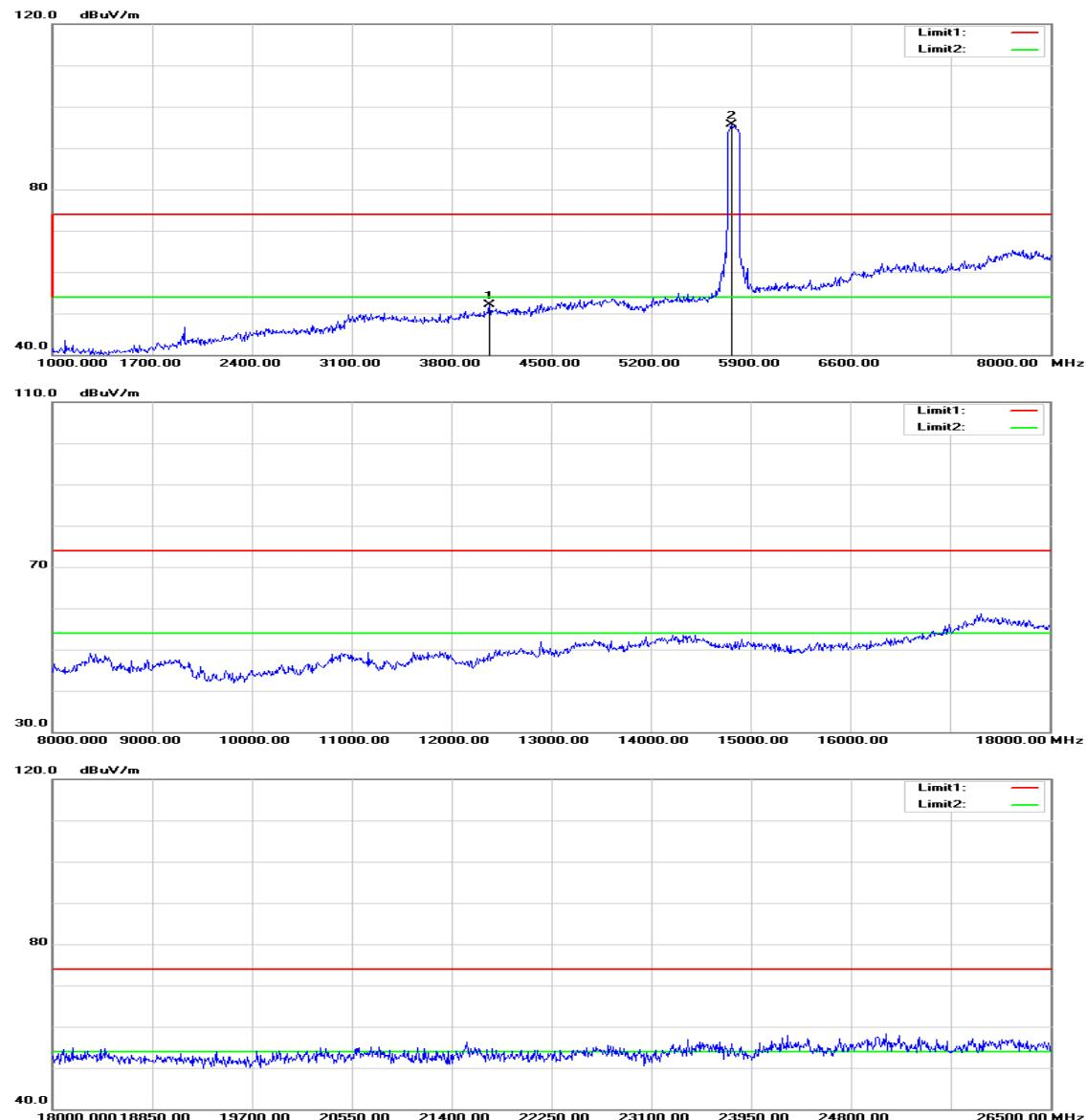
**Operation Mode:** Tx / IEEE 802.11ac VHT 80 MHz mode / 5775MHz**Test Date:** July 31, 2015**Temperature:** 27°C**Tested by:** Owen Wu**Humidity:** 53% RH**Polarity:** Ver. / Hor.
