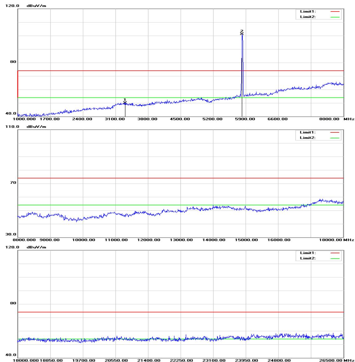
**Operation Mode:** TX / IEEE 802.11a mode / 5825MHz**Test Date:** July 31, 2015**Temperature:** 27°C**Tested by:** Owen Wu**Humidity:** 53% RH**Polarity:** Ver. / Hor.
