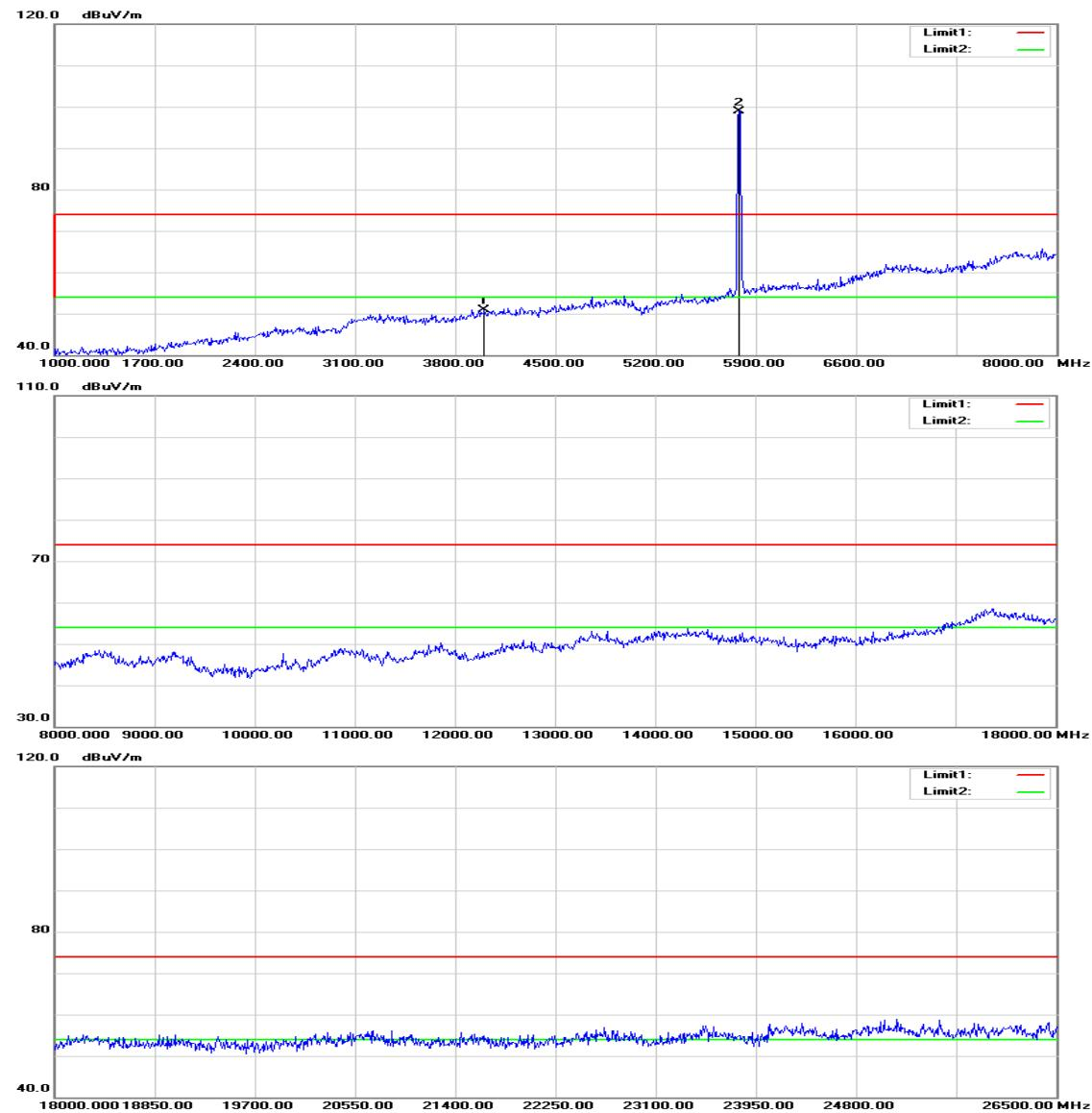
**Operation Mode:** TX / IEEE 802.11a mode / 5785MHz**Test Date:** July 31, 2015**Temperature:** 27°C**Tested by:** Owen Wu**Humidity:** 53% RH**Polarity:** Ver. / Hor.
