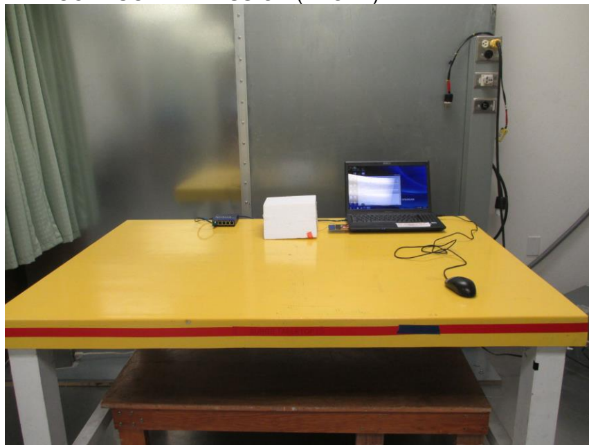
LINE CONDUCTED EMISSION (FRONT)
