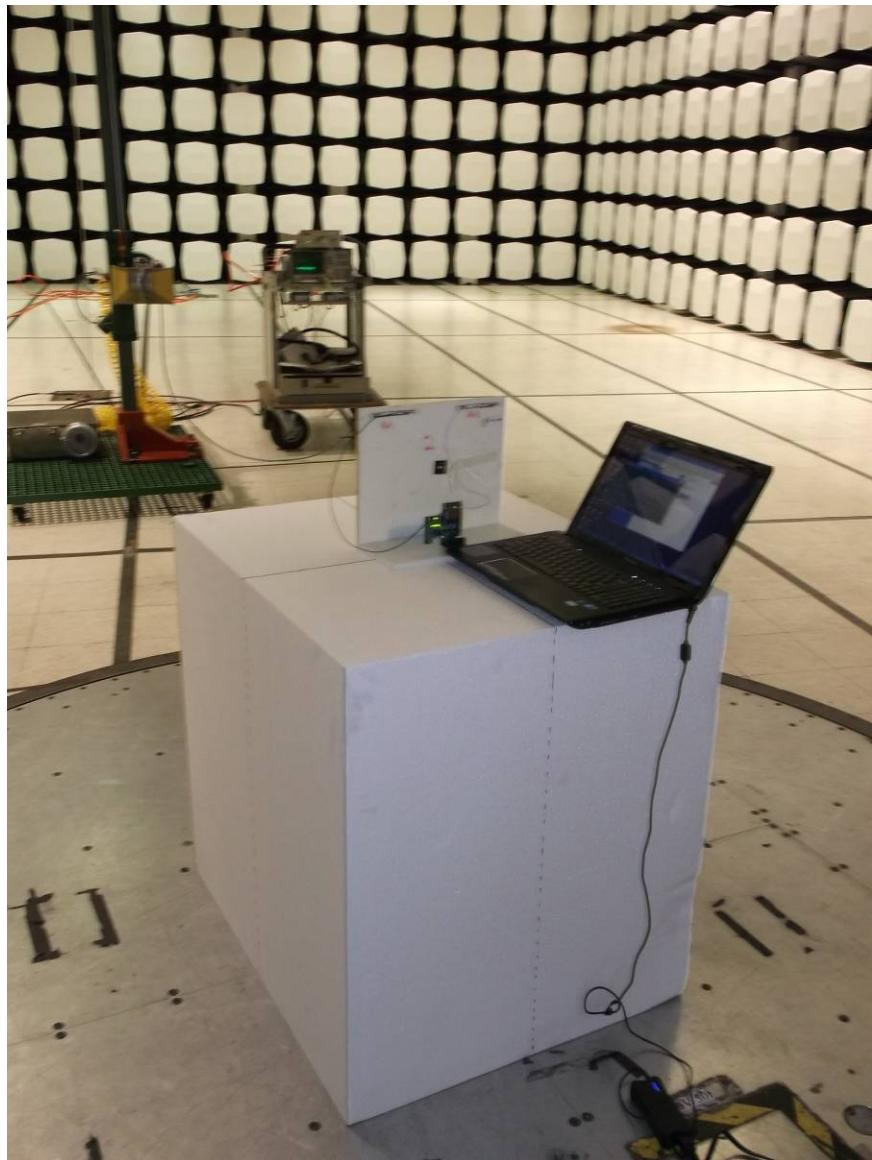
*CONDUCTED EMISSIONS TEST CONFIGURATION PHOTOGRAPHS*
