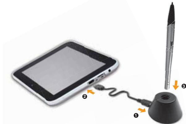
The digitizer pen is not fully charged at purchase. Charge the digitizer pen before using it for the first time. To charge the digitizer pen, do the following:
