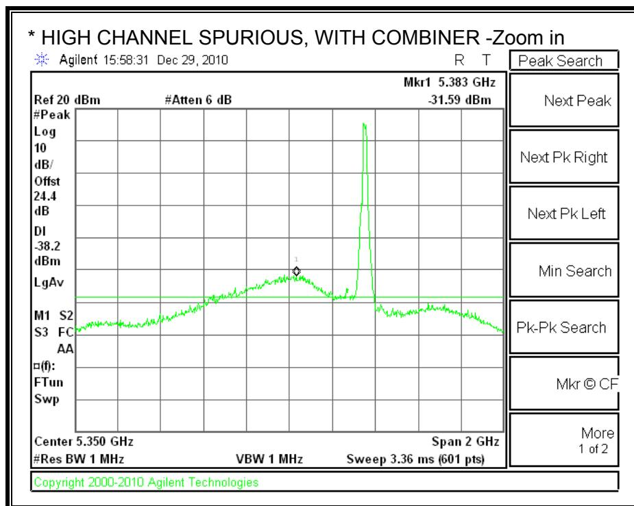
\* Passed with EIRP Radiated Substitution
