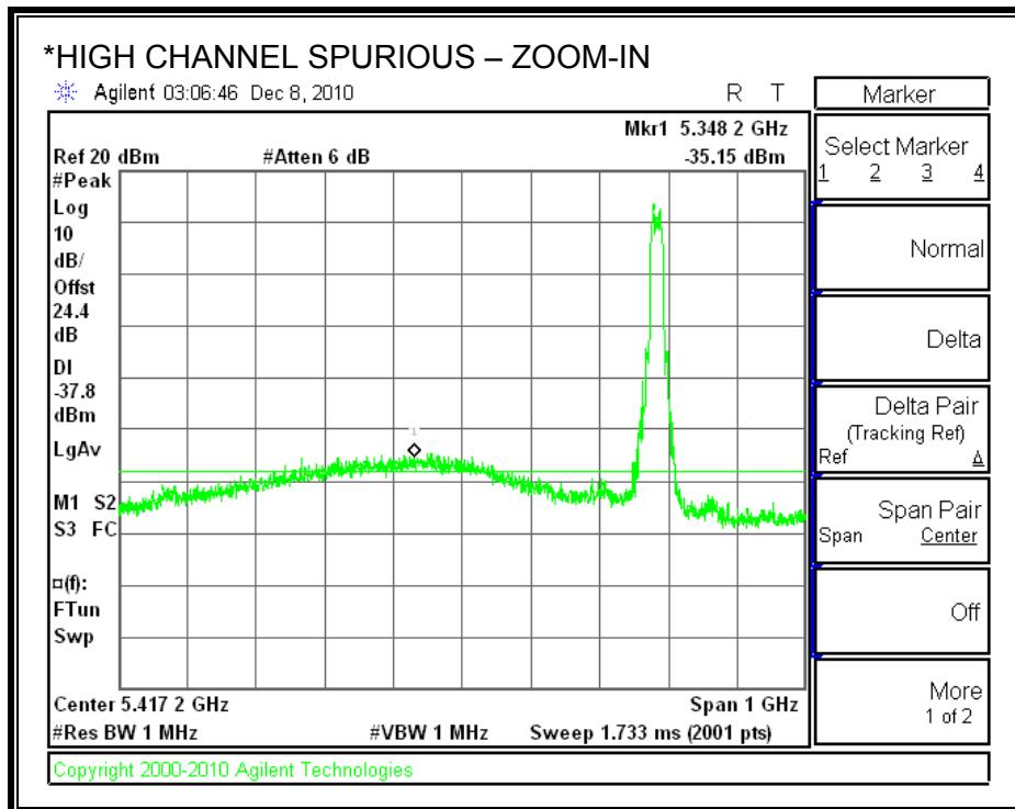
\* Passed with EIRP Radiated Substitution
