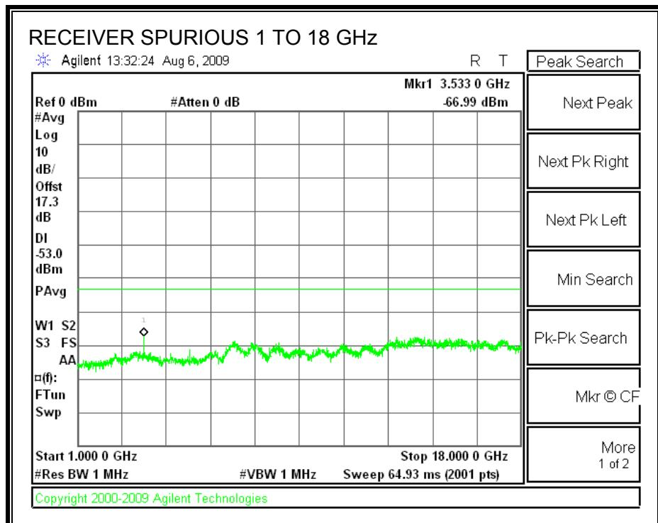
**RECEIVER SPURIOUS EMISSIONS IN THE 5.5 GHz BAND**
