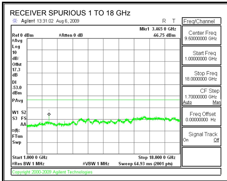
**RECEIVER SPURIOUS EMISSIONS IN THE 5.3 GHz BAND**
