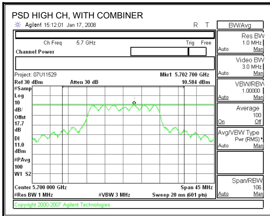
**POWER SPECTRAL DENSITY WITH COMBINER (7.21 dBi Antenna Gain)**
