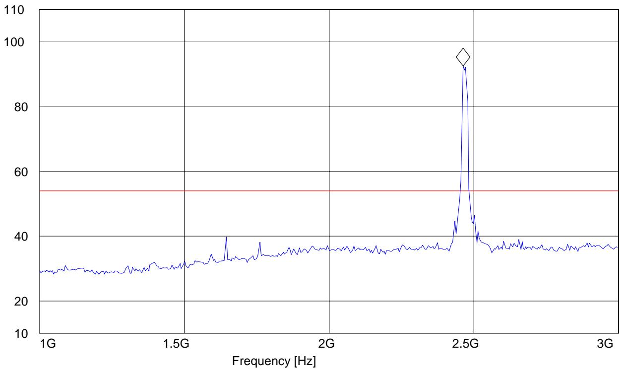
**1-3GHz (2467MHz, Ch 12) Antenna Vertical**
