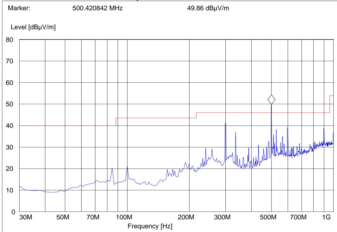
**30MHz – 1GHz, Antenna: Horizontal****Note: This plot is valid for channels 12 and 13 (worst-case plot).****Note: Emissions over the limits are caused by the test fixture and the laptop. This is demonstrated by removing of the module and the emissions persist. See plots on next page.**
