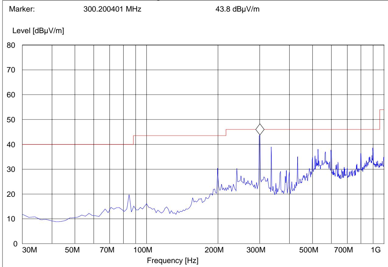
**30MHz – 1GHz, Antenna: Vertical with EUT removed.
