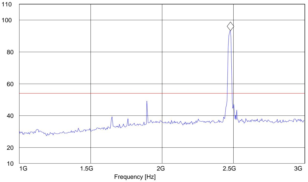
**1-3GHz (2472MHz Ch13) Antenna Vertical**
