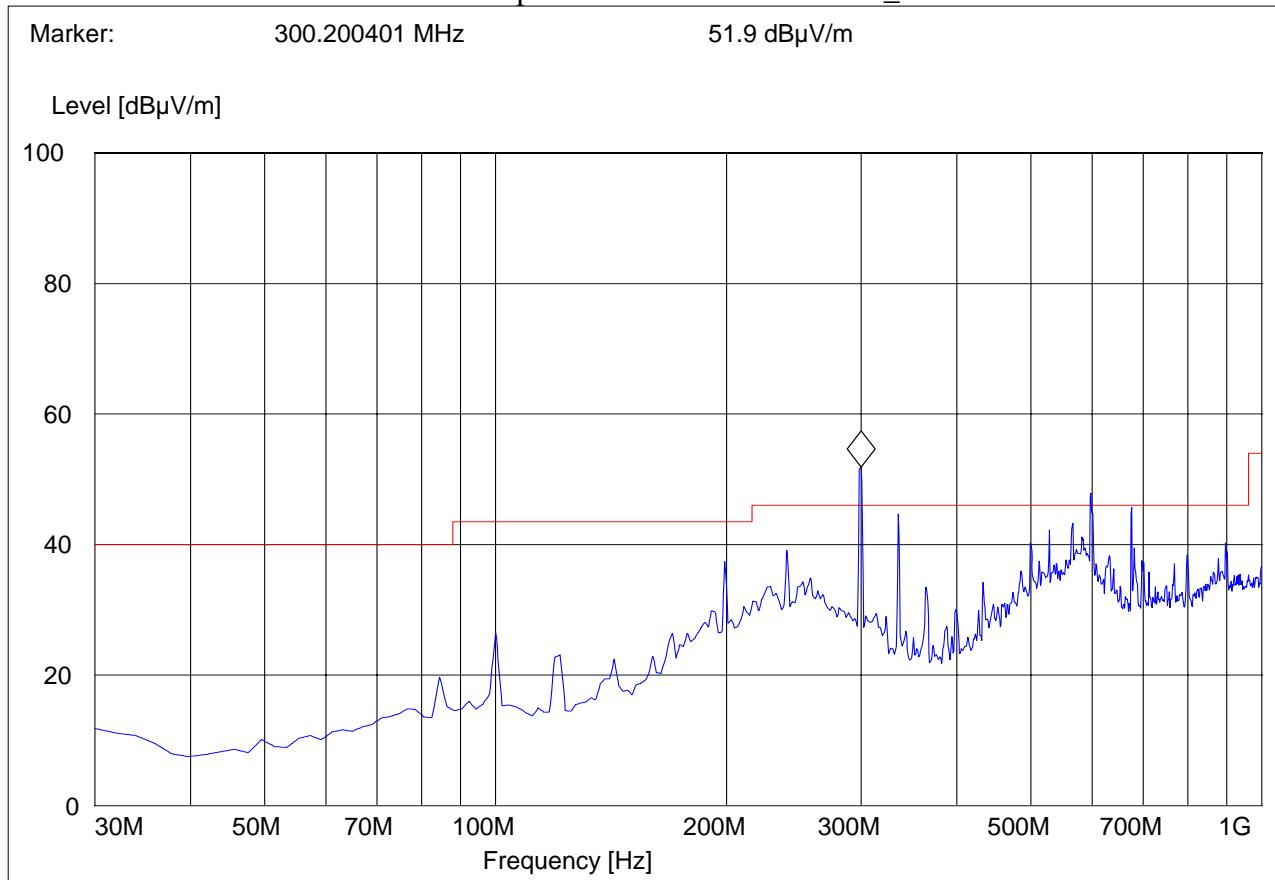
**30MHz – 1GHz, Antenna: Horizontal with EUT removed.****Test fixture and supporting laptop only.**
