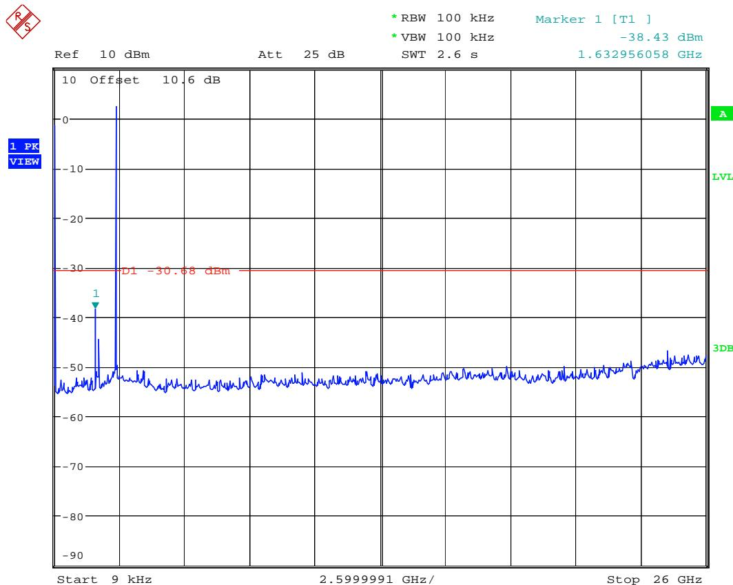
**Conducted Emission Ch13 802.11b****Emission over the limit line is Tx wanted emission.**
