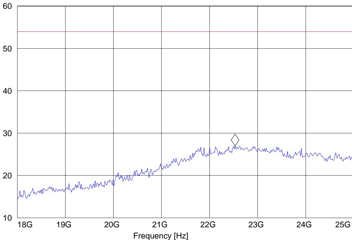
**5.8 EMISSION LIMITATIONS – Radiated (Receiver)****RSS-GEN (4.10) & (6):****Limits RSS-GEN (4.10) & (6):**
