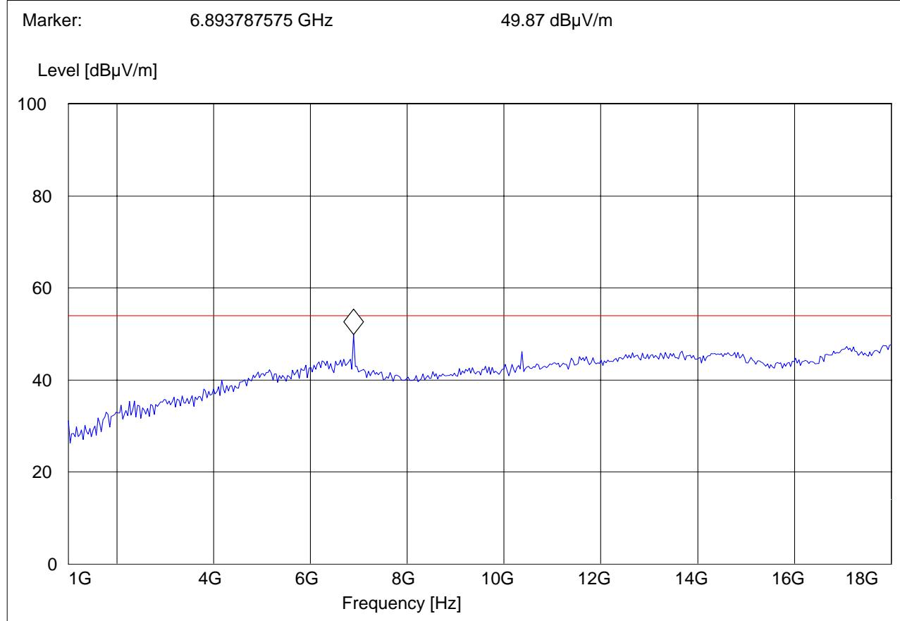
**1-18GHz (5320MHz)****Note: The peaks above the limit line is the carrier freq.****Note: Peak Reading vs. Average limit (54 dB $\mu$ V/m)**
