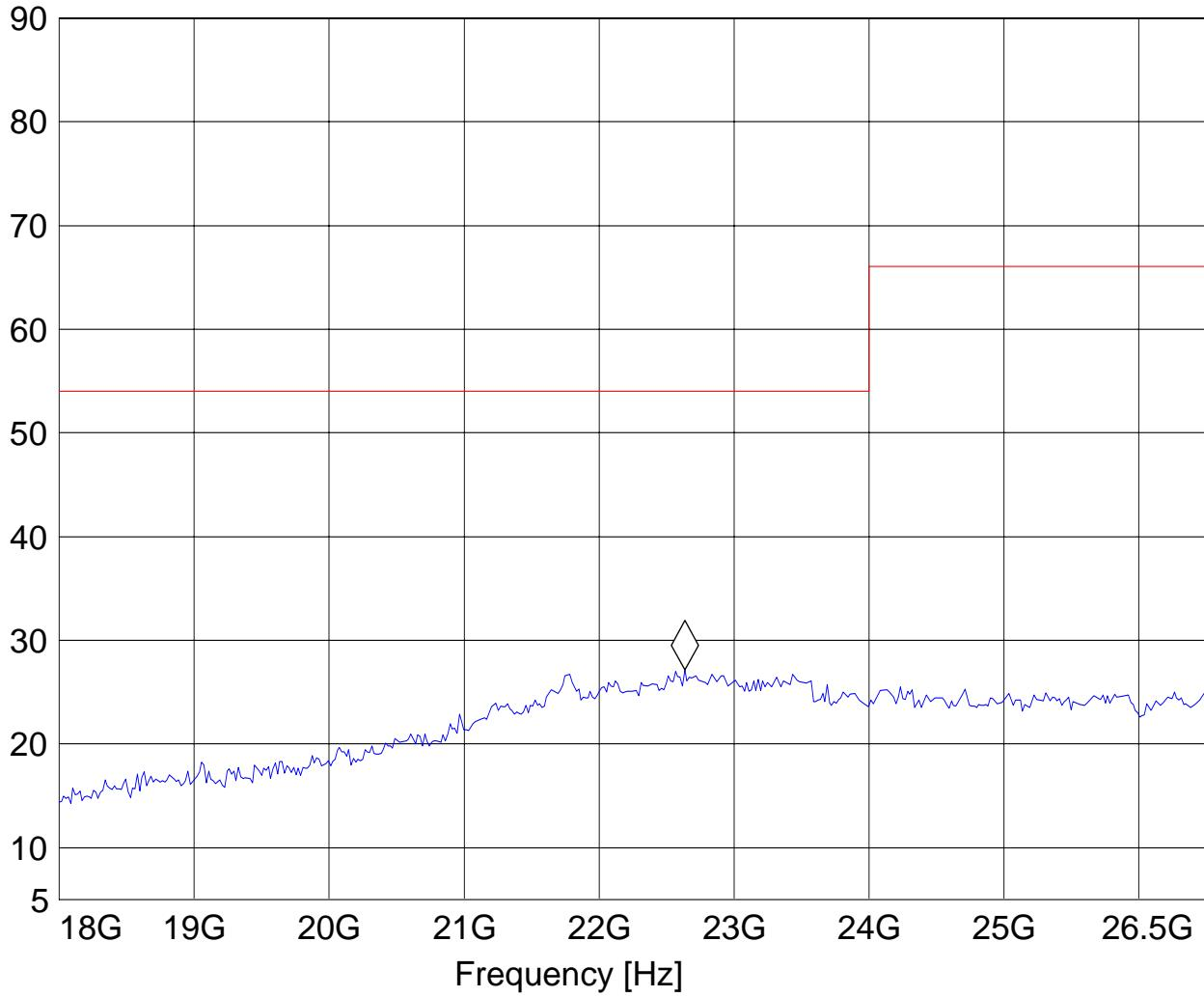
**18-26.5GHz (5260MHz)****Note: Peak Reading vs. Average limit (54 dB $\mu$ V/m)****CETECOM Inc., 411 Dixon Landing Road, Milpitas CA 95035, USA**
