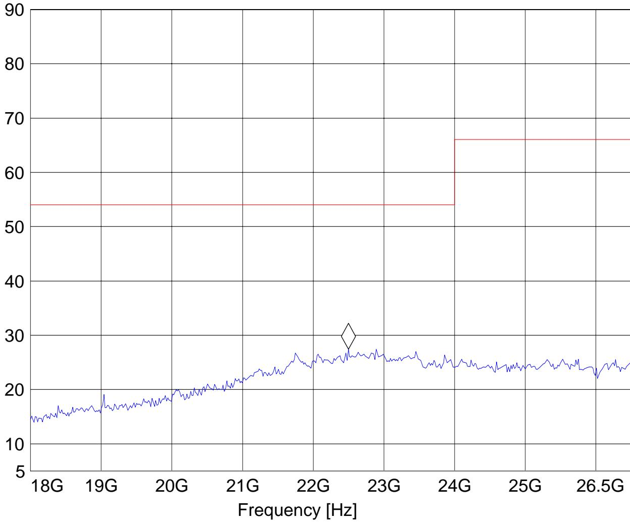
**18-26.5GHz (5320MHz)****Note: Peak Reading vs. Average limit (54 dB $\mu$ V/m)****CETECOM Inc., 411 Dixon Landing Road, Milpitas CA 95035, USA**
