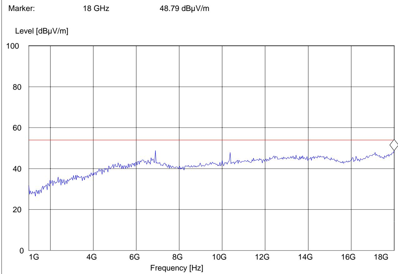
**1-18GHz (5260MHz)****Note: The peaks above the limit line is the carrier freq.****Note: Peak Reading vs. Average limit (54 dBuV/m)**
