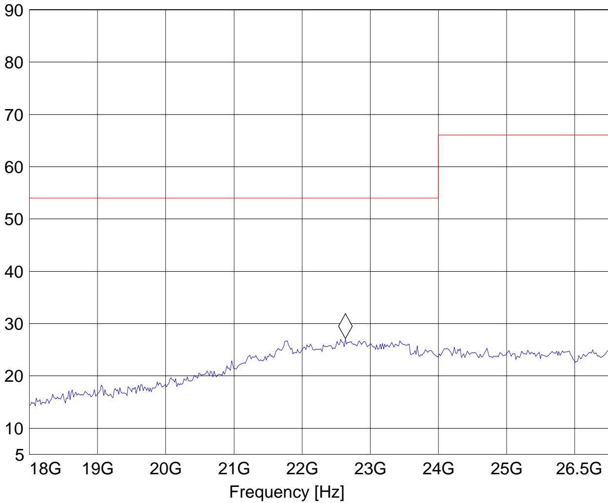
**18-26.5GHz (5260MHz)****Note: Peak Reading vs. Average limit (54 dB $\mu$ V/m)**
