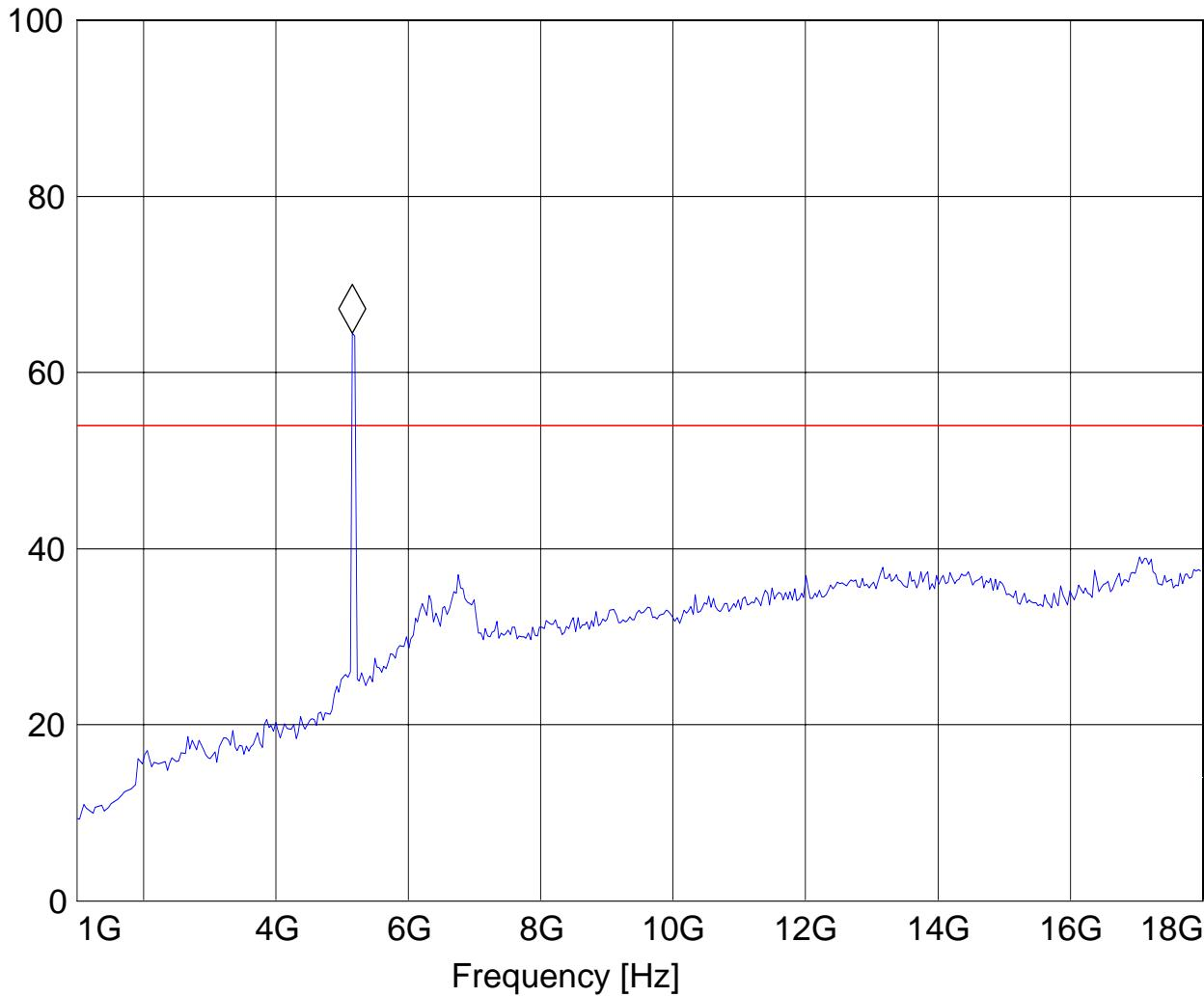
**1-18GHz (5260MHz)****Note: The peaks above the limit line is the carrier freq.****Note: Peak Reading vs. Average limit (54 dB $\mu$ V/m)**
