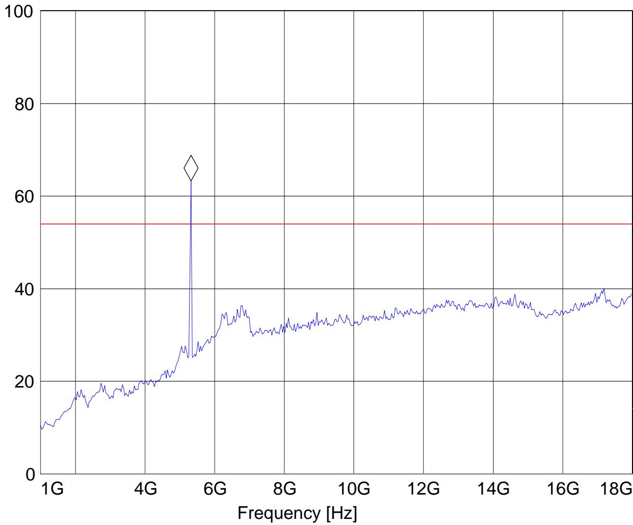
**18-26.5GHz (5180MHz)****Note: Peak Reading vs. Average limit (54 dB $\mu$ V/m)**
