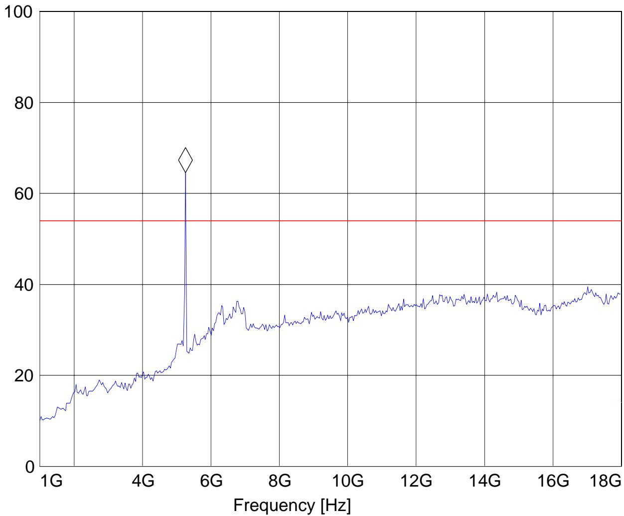
**1-18GHz (5320MHz)****Note: The peaks above the limit line is the carrier freq.****Note: Peak Reading vs. Average limit (54 dB $\mu$ V/m)**
