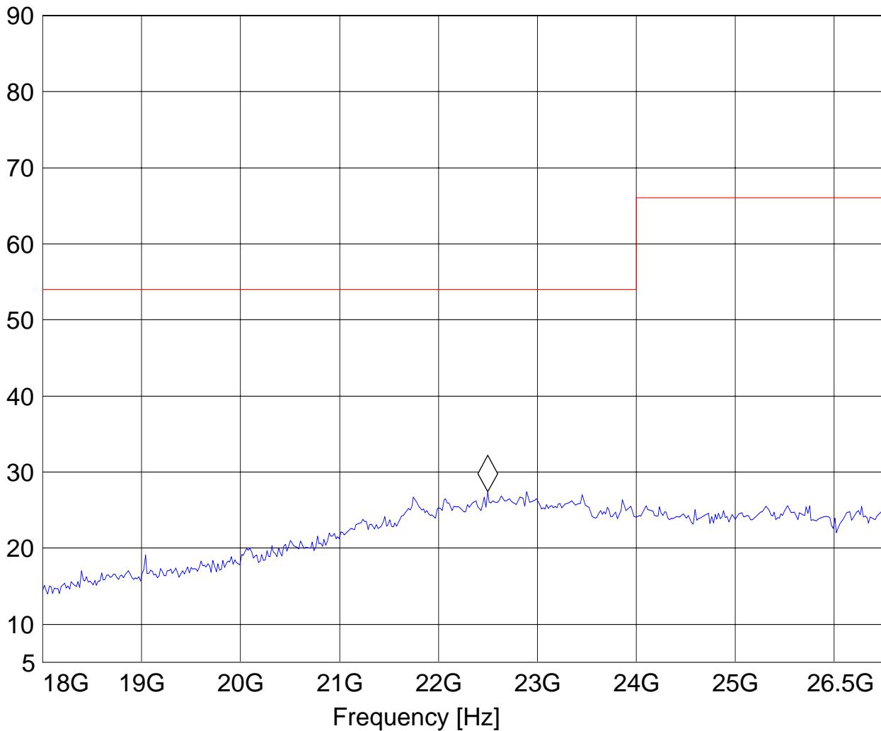
**18-26.5GHz (5320MHz)****Note: Peak Reading vs. Average limit (54 dB $\mu$ V/m)**
