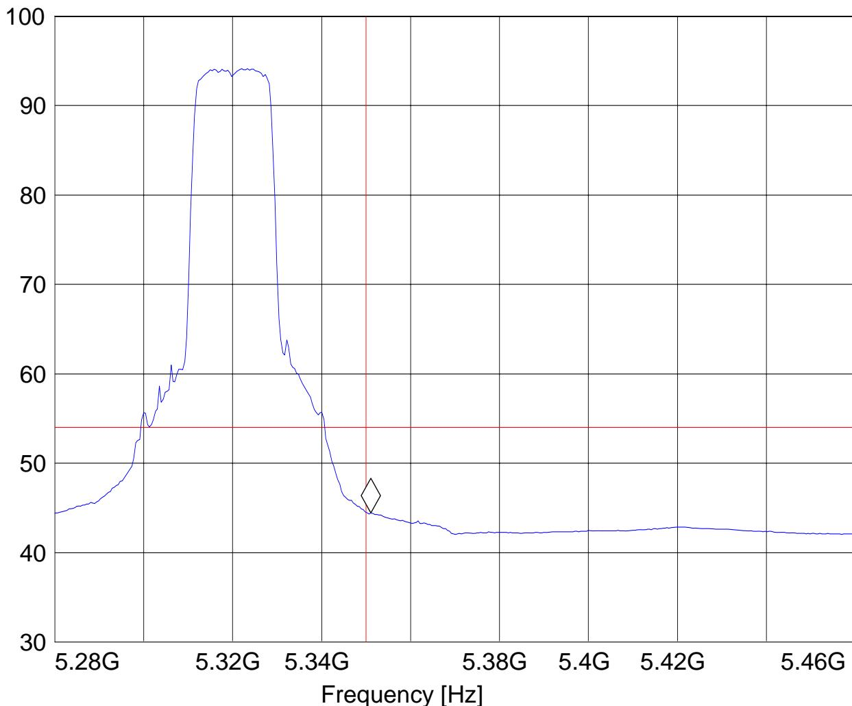
**5.3 TRANSMITTER SPURIOUS EMISSIONS RADIATED § 15.407(b)/15.205/15.209****5.3.1 LIMITS**
