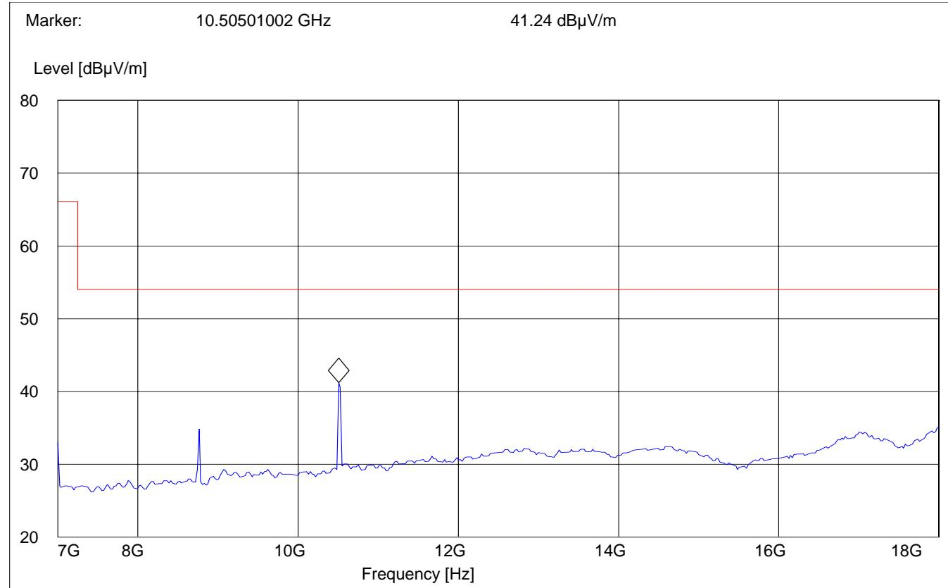
**EMISSION LIMITATIONS - Radiated (Transmitter)****§ 15.407 (b)(1)(2)(4)(6)****Highest Channel (5320MHz): 1GHz – 7GHz****(Average)****Antenna:** Horizontal**EUT plane:** Horizontal with screen vertical @ 90°**Note: The peak above the limit line is the carrier freq.**
