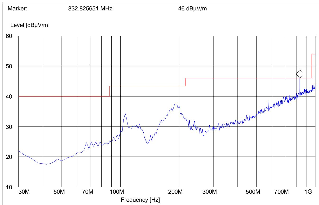
**EMISSION LIMITATIONS - Radiated (Transmitter)****§ 15.407 (b)(1)(2)(4)(6)****Lowest Channel (5180MHz): 1GHz – 7GHz****(Average)****Antenna:** Horizontal**EUT plane:** Horizontal with screen vertical @ 90°**Note: The peak above the limit line is the carrier freq.**
