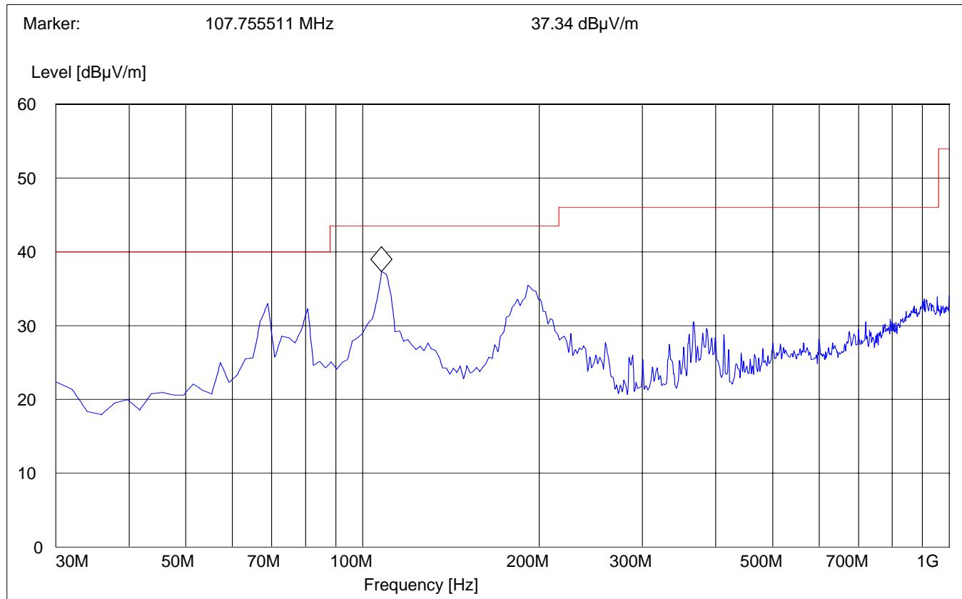
**EMISSION LIMITATIONS - Radiated (Transmitter)****§ 15.407 (b)(1)(2)(4)(6)****Lowest Channel (5180MHz): 30MHz – 1GHz**
