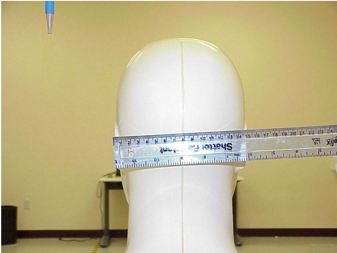
Photo 12. Photo to demonstrate 15 cm Z-axis head phantom
