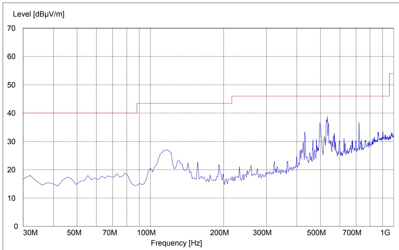
**EMISSION LIMITATIONS - Radiated (Transmitter)****§ 15.247 (c) (1)****Lowest Channel (2412MHz): 1GHz – 3GHz****Average Measurement****SWEEP TABLE: "BT Spuri hi 1-3G"**
