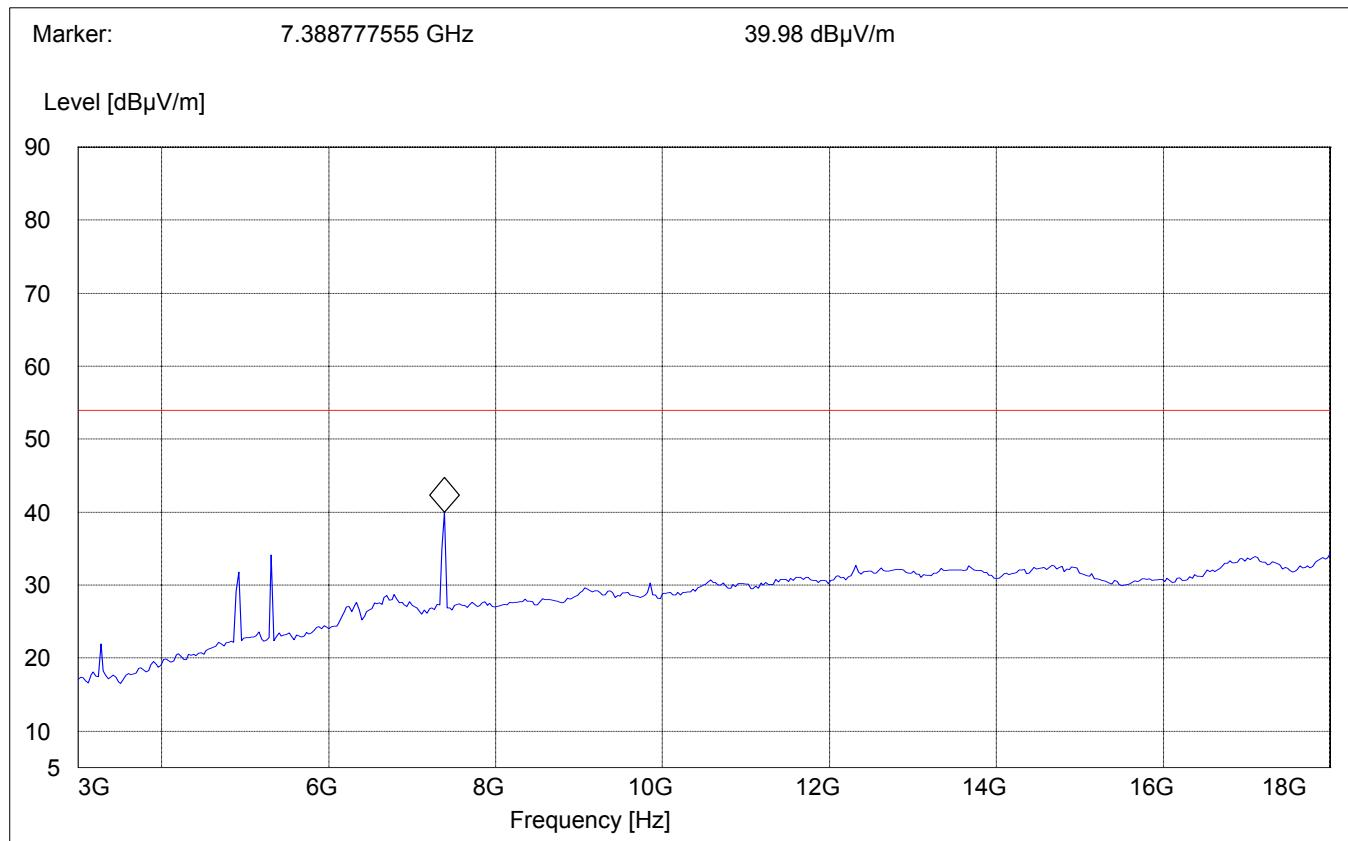
**EMISSION LIMITATIONS - Radiated (Transmitter)**      **§ 15.247 (c) (1)**
