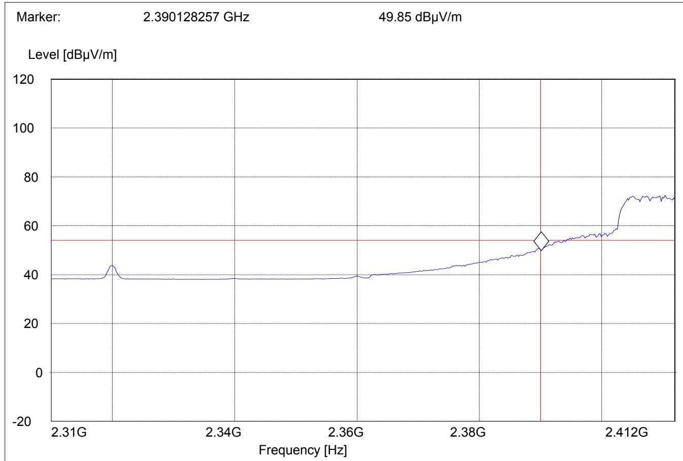
**BAND EDGE COMPLIANCE****§15.247 (c)****Low frequency section (spurious in the restricted band 2310 – 2390 MHz)****(Peak measurement)**
