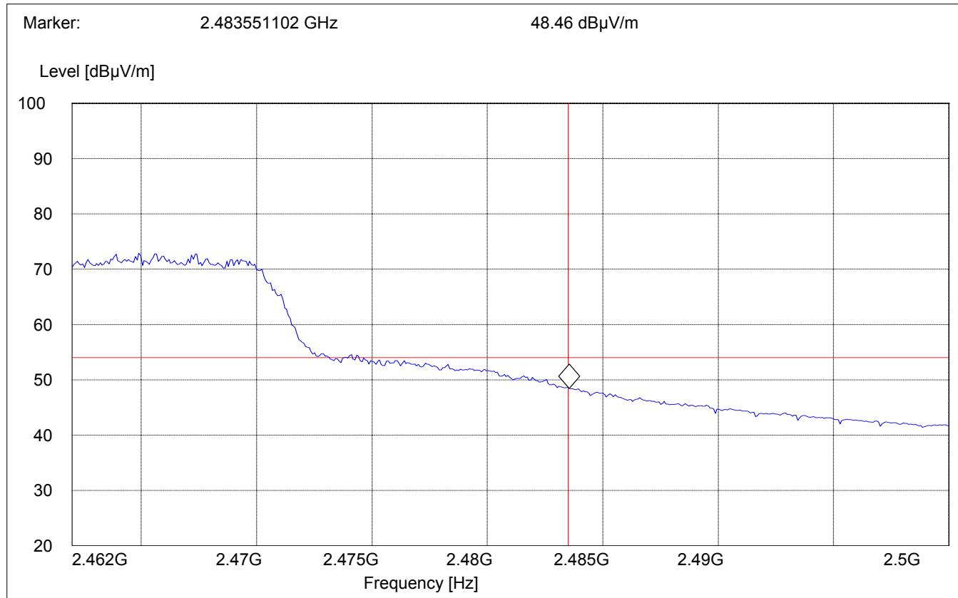
**BAND EDGE COMPLIANCE****§15.247 (c)****High frequency section (spurious in the restricted band 2483.5 – 2500 MHz)
