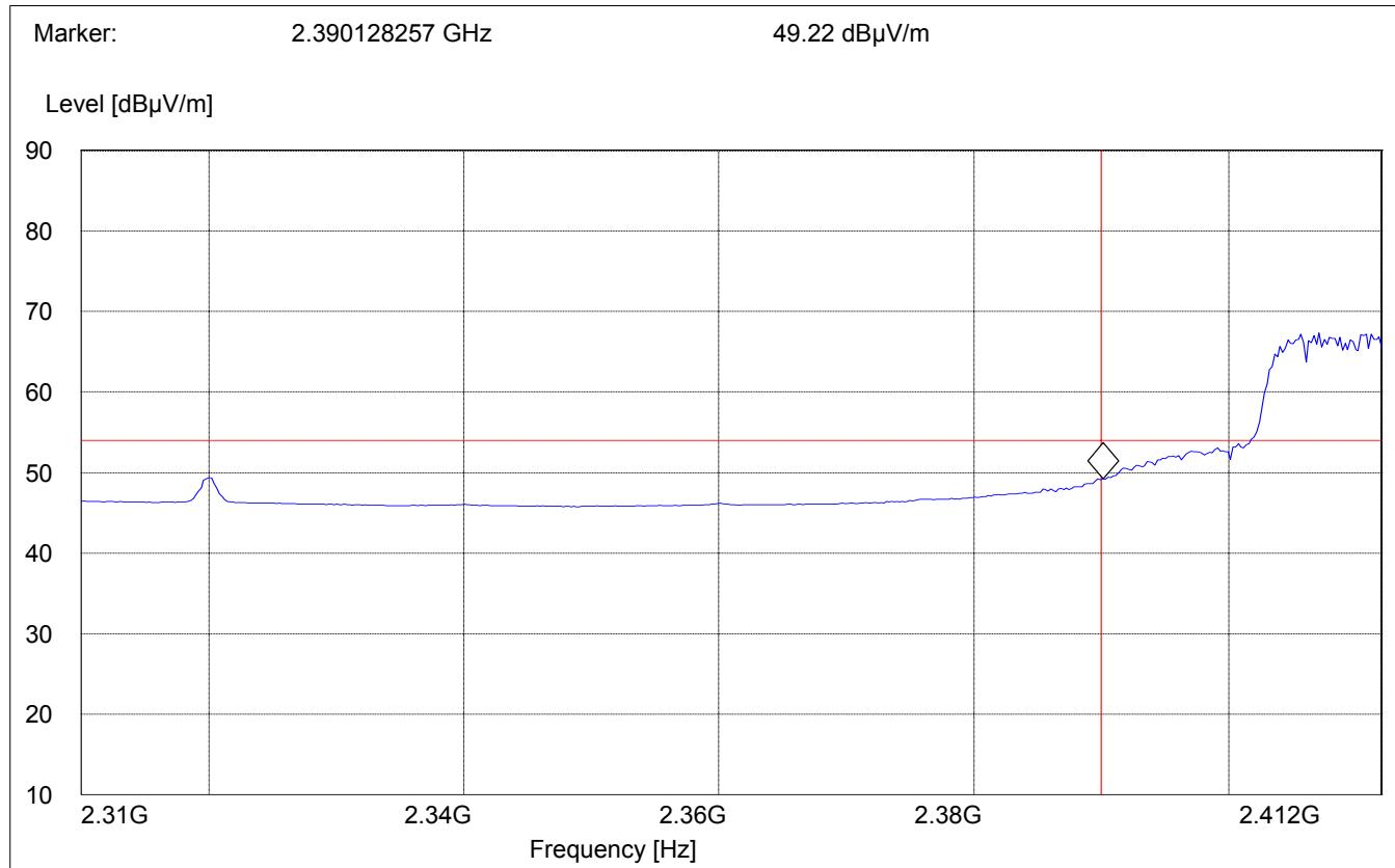
**BAND EDGE COMPLIANCE****§15.247 (c)****Low frequency section (spurious in the restricted band 2310 – 2390 MHz)****(Peak measurement)**
