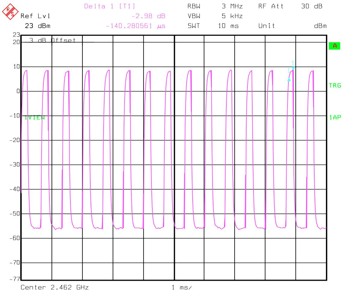
Transmitter ON+OFF time –  $T_{x_{on}} + T_{x_{off}}$
