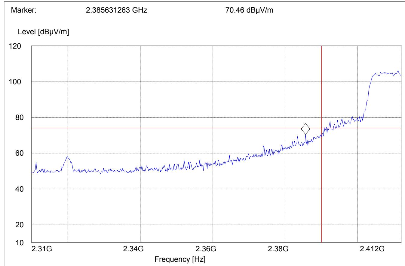
**BAND EDGE COMPLIANCE****§15.247 (c)****High frequency section (spurious in the restricted band 2483.5 – 2500 MHz)****(Average measurement)**
