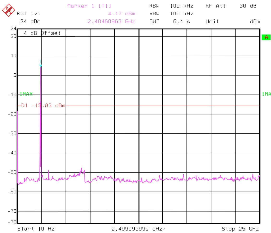
**EMISSION LIMITATIONS - Conducted (Transmitter)****§ 15.247 (c) (1)****Mid Channel (2437MHz): 10MHz - 25GHz**
