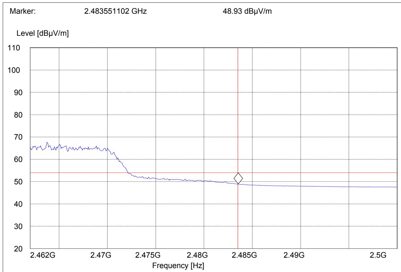
**BAND EDGE COMPLIANCE****§15.247 (c)****High frequency section (spurious in the restricted band 2483.5 – 2500 MHz)
