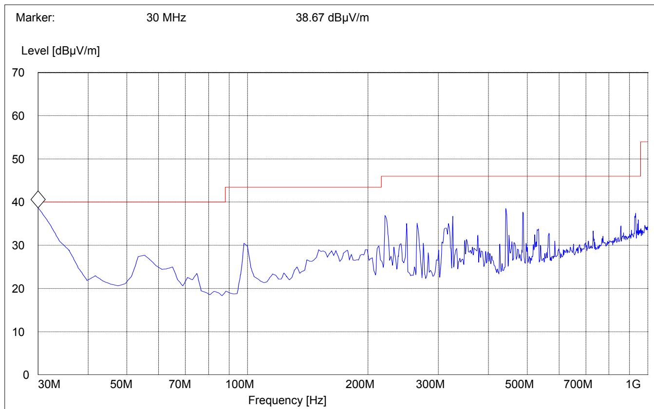
**EMISSION LIMITATIONS - Radiated (Transmitter)****§ 15.247 (c) (1)****Highest Channel (2462MHz): 1GHz – 3GHz****Average Measurement with VBW=10Hz****(Bluetooth Module Tx @ Mid channel)**
