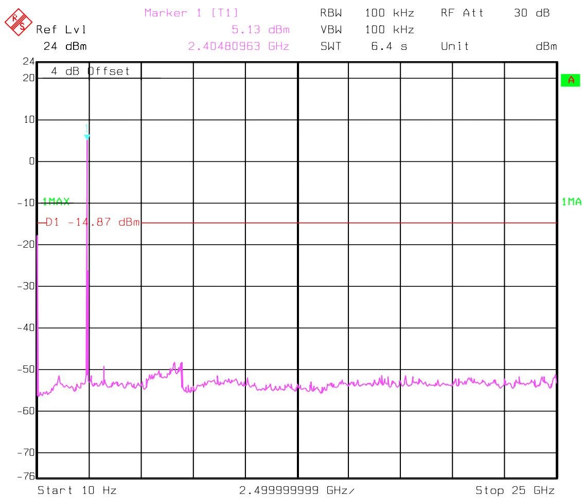
**EMISSION LIMITATIONS - Conducted (Transmitter)****§ 15.247 (c) (1)****Highest Channel (2462MHz): 10MHz - 25GHz**
