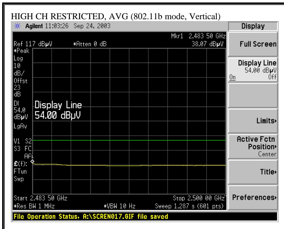
**HARMONICS AND SPURIOUS EMISSIONS (b MODE, LOW CHANNEL), TRANSMIT**
