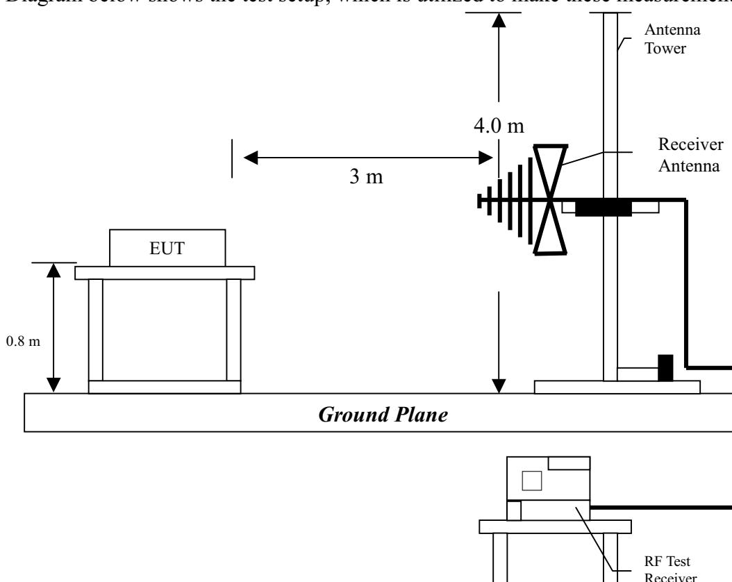
Radiated emission measurements were performed from 30MHz to 25GHz. Spectrum Analyzer Resolution Bandwidth is 100kHz or greater for frequencies 30MHz to 1GHz, 1MHz – for frequencies above 1GHz.
