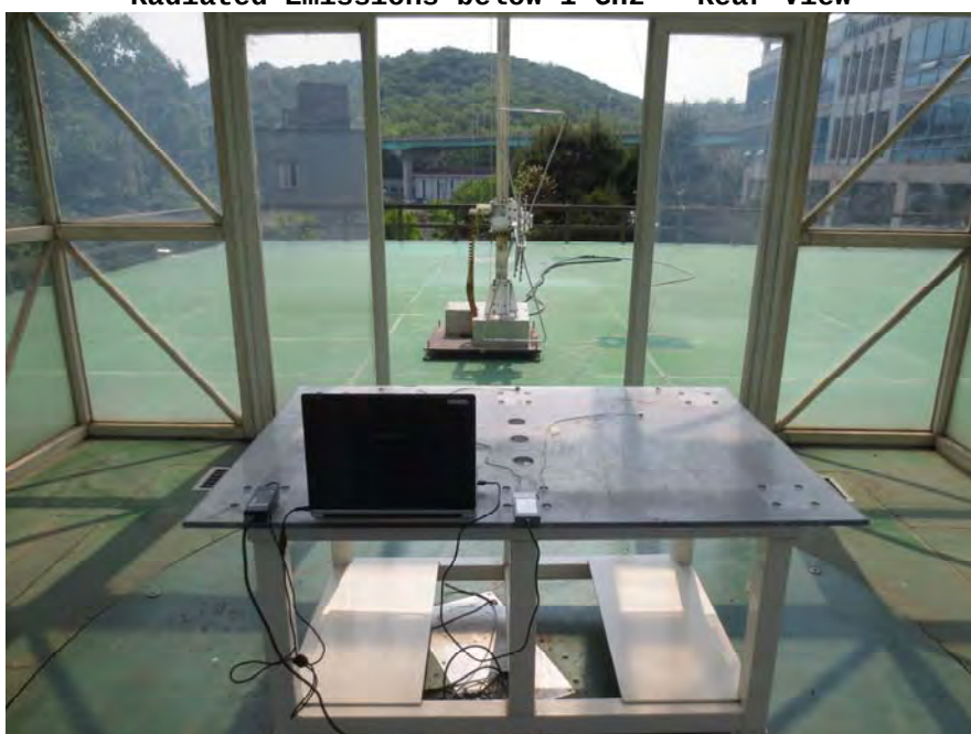
Radiated Emissions below 1 GHz - Rear View
