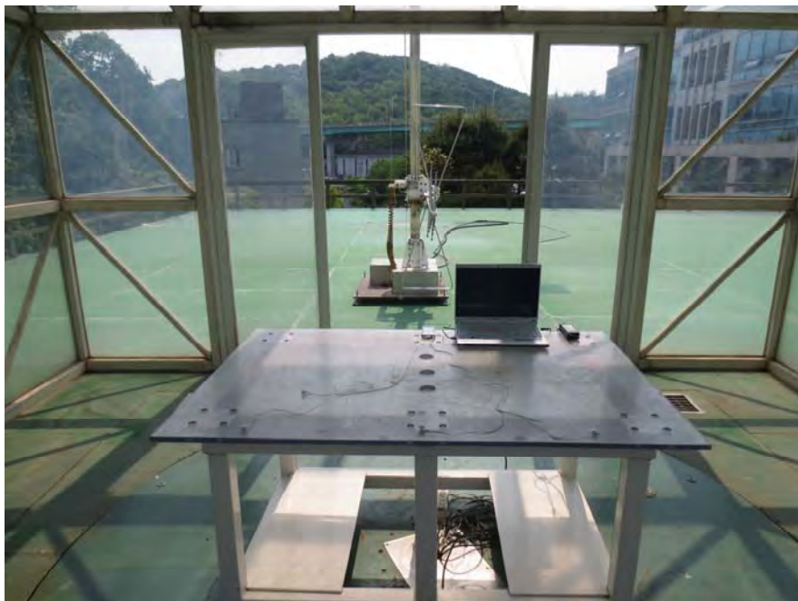
Radiated Emissions below 1 GHz - Rear View
