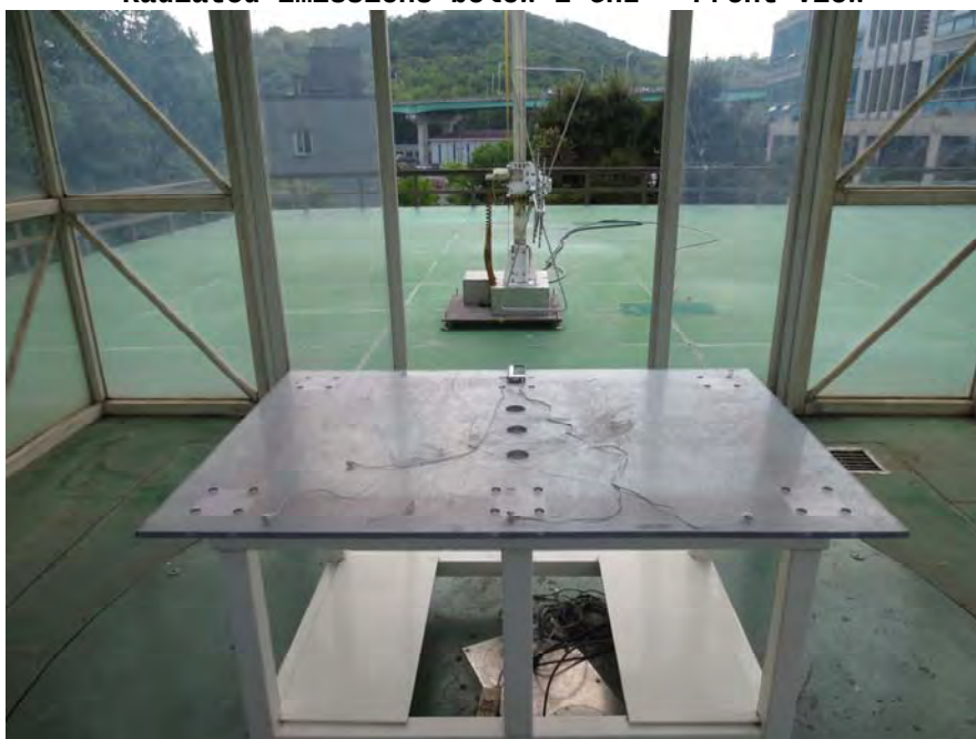
Radiated Emissions below 1 GHz - Rear View
