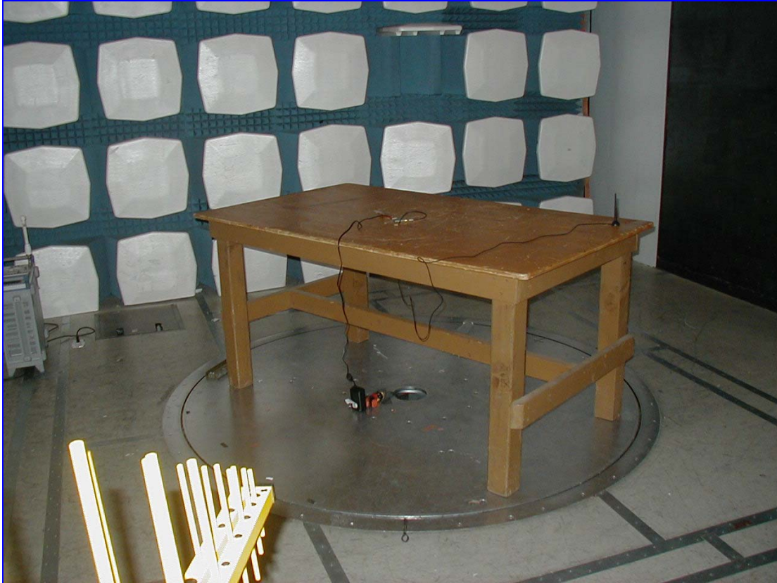
Photograph 1. Unintentional Radiated Emission Limits, Test Setup
