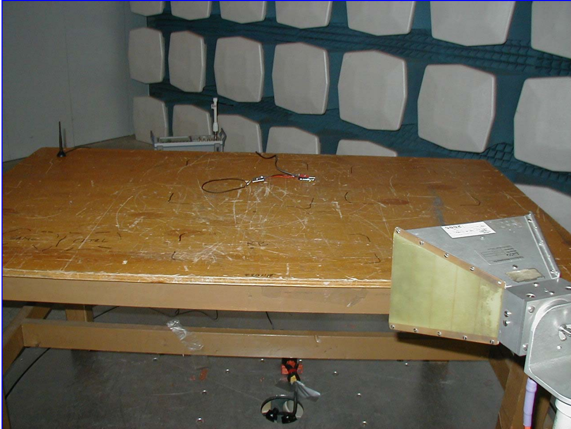
Photograph 3. Unintentional Radiated Emission Limits, Test Setup
