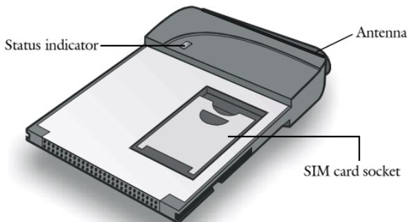
Move the antenna upward while in use.
