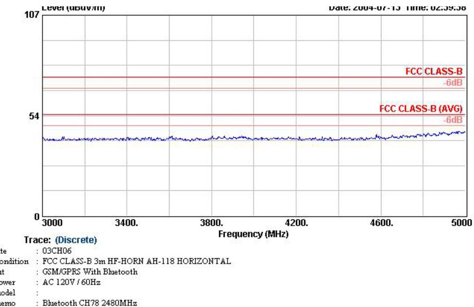
Remark: Frequency from 5000MHz to 25000MHz, the emission emitted by the EUT is too low to be measured.
