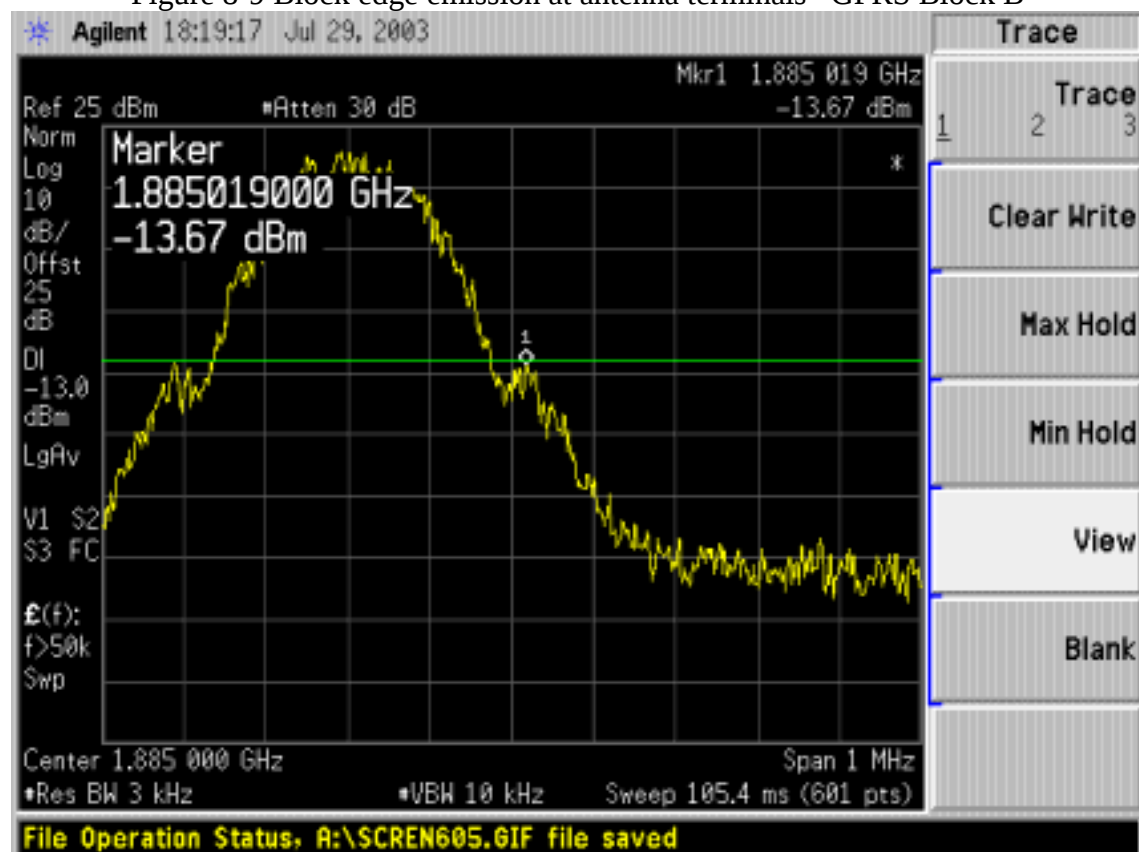
Figure 8-9 Block edge emission at antenna terminals –GPRS Block B
