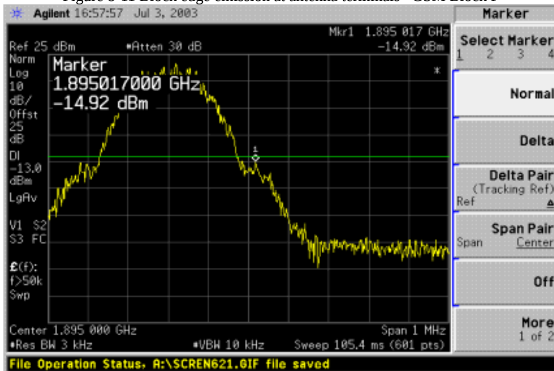
Figure 8-11 Block edge emission at antenna terminals –GSM Block F
