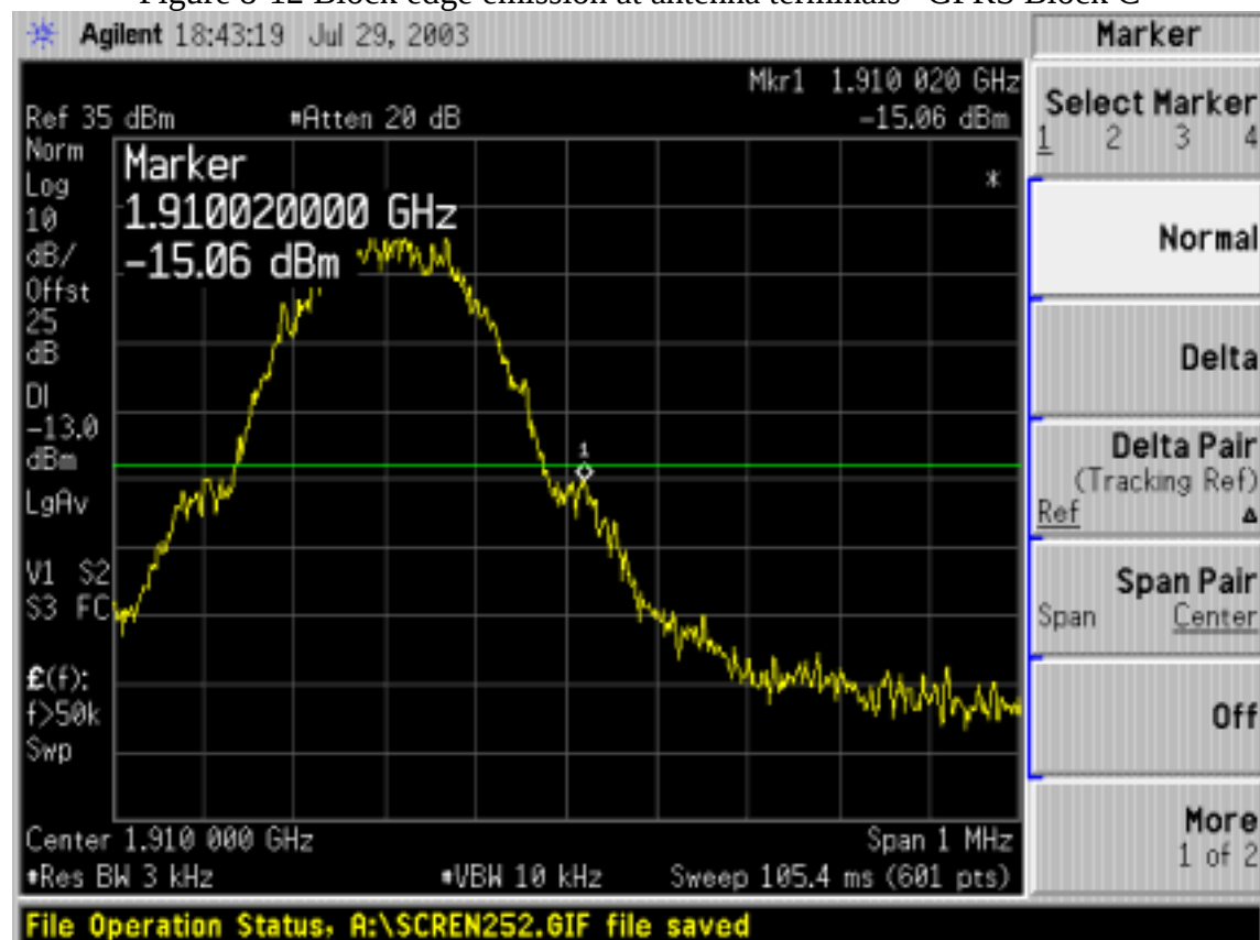
Figure 8-12 Block edge emission at antenna terminals –GPRS Block C
