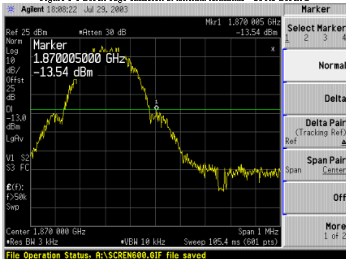
Figure 8-8 Block edge emission at antenna terminals –GPRS Block D
