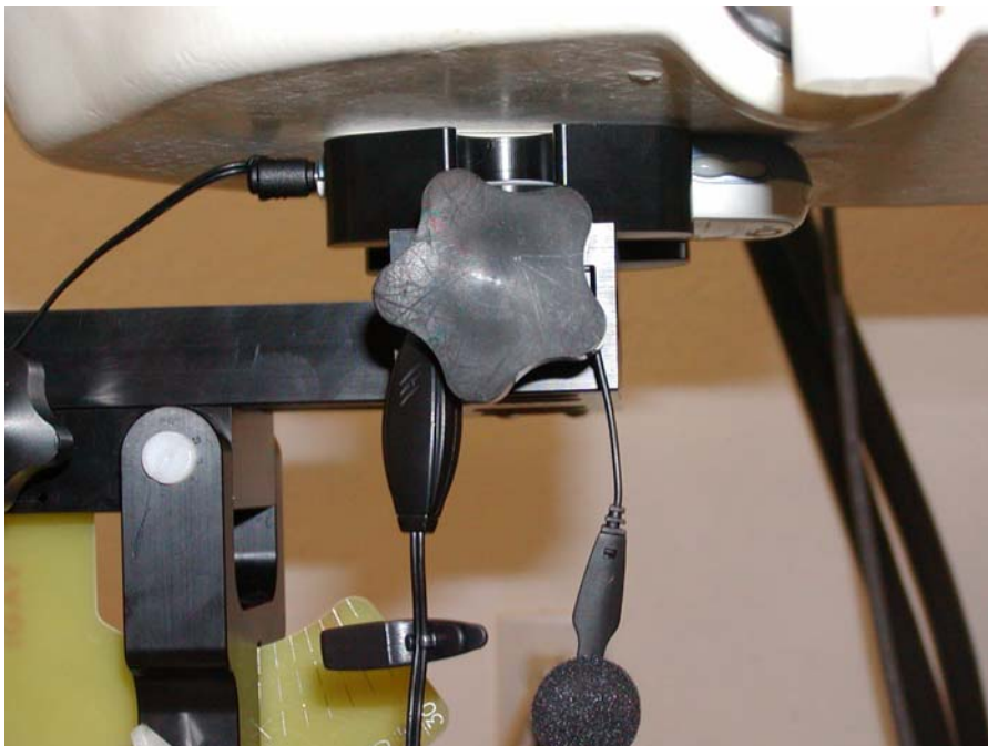
Bottom Touching Phantom with Earphone – Side View
