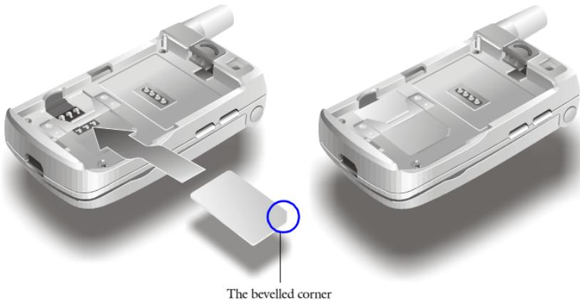
Pay special attention to the SIM card when you install and remove. Its metal contact can be damaged easily by scratches.
