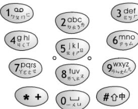
The alphanumeric keys on the phone can be used to enter numbers and letters. To enter phone numbers, press corresponding number keys directly. To enter letters, please see "Entering text" on page 22 for details.
