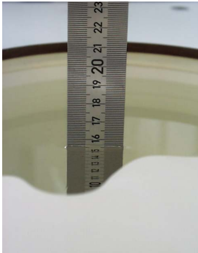
Fig. 24 :Liquid depth for Head measurements.
