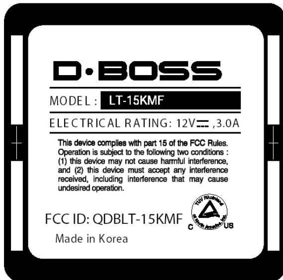
**■ ID Label Location of EUT****I.D Label**
