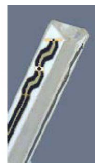
Figure 3.3 Probe Thick-Film Technique
