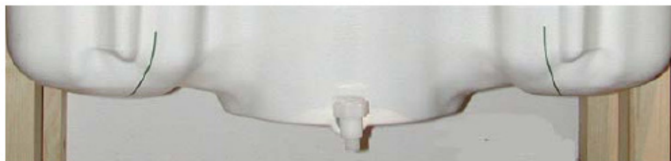
Figure 7.2 SAM Twin Phantom shell
