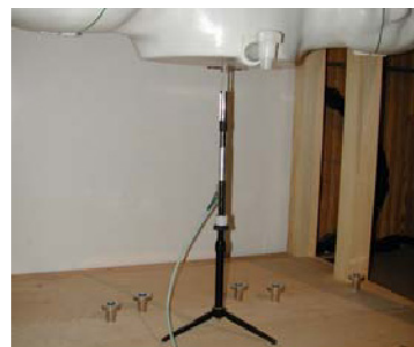
Figure 12.1 Dipole Validation Test Setup
