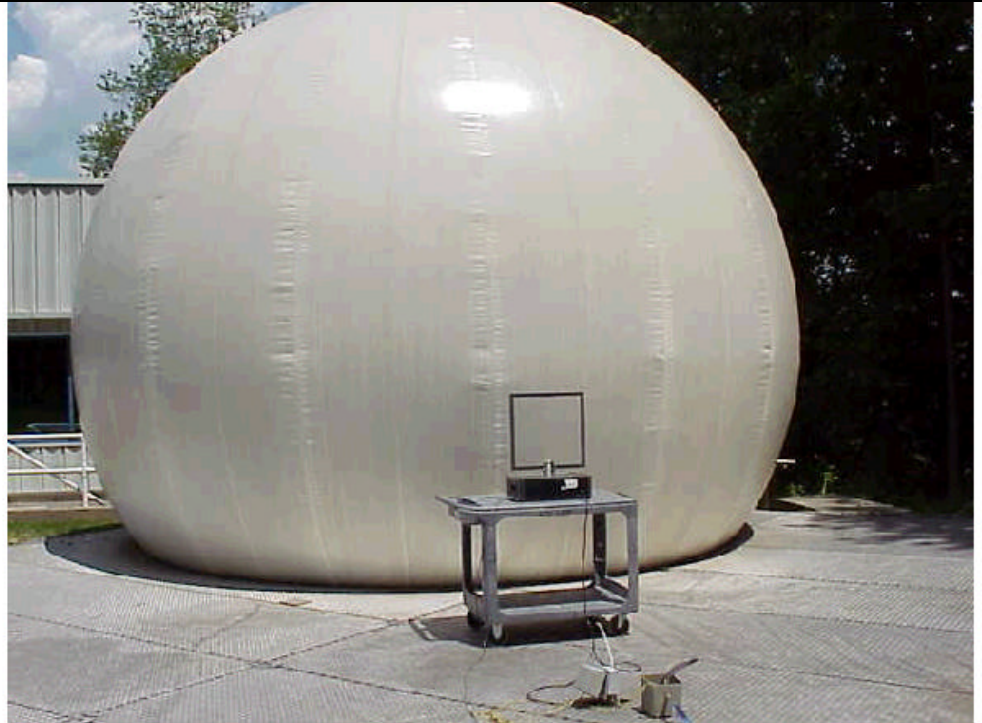
Radiated Emissions Open Area Test Site (OATS) for 100 kHz to 30MHz at 3 meters
