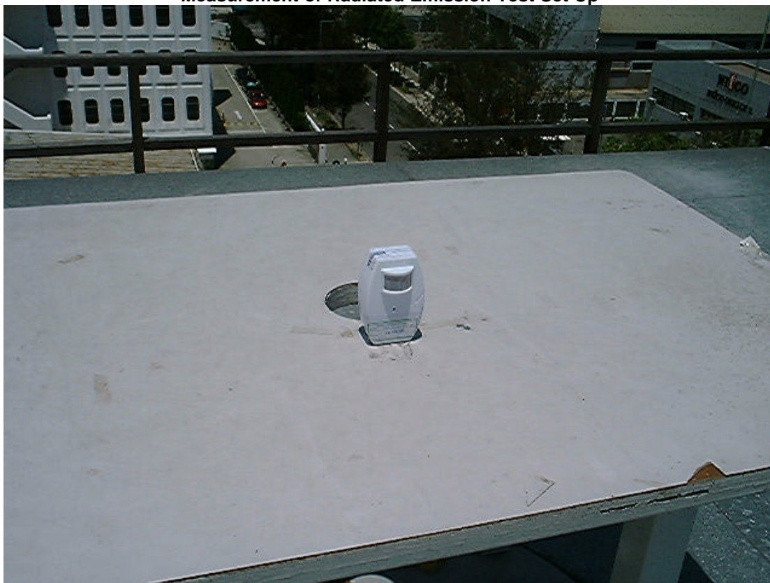
Measurement of Radiated Emission Test Set Up
